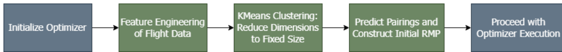
Figure 3.10: Summary of the integration of GEPI into Boeing’s optimizer. The steps highlighted in green represent the new procedures introduced by GEPI, while the blue boxes indicate the original steps in Boeing’s optimizer’s workflow.
