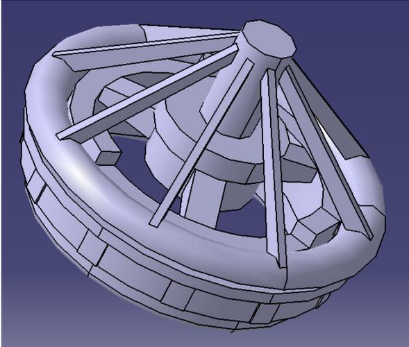
*Figure 16. The customized frame mold for the injection molding phase when injecting the sealing material, created in Catia V5*
