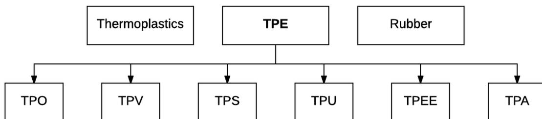
Figure 2. The different variations in the TPE material group, Adapted with permission from Hexpol
