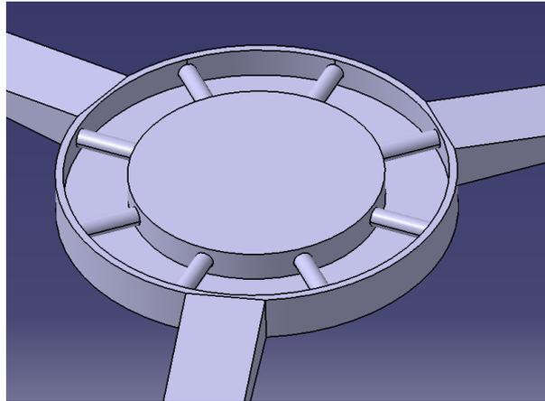
*Figure 9. A Catia V5 model for the initial idea for concept 2's mechanical lock*
