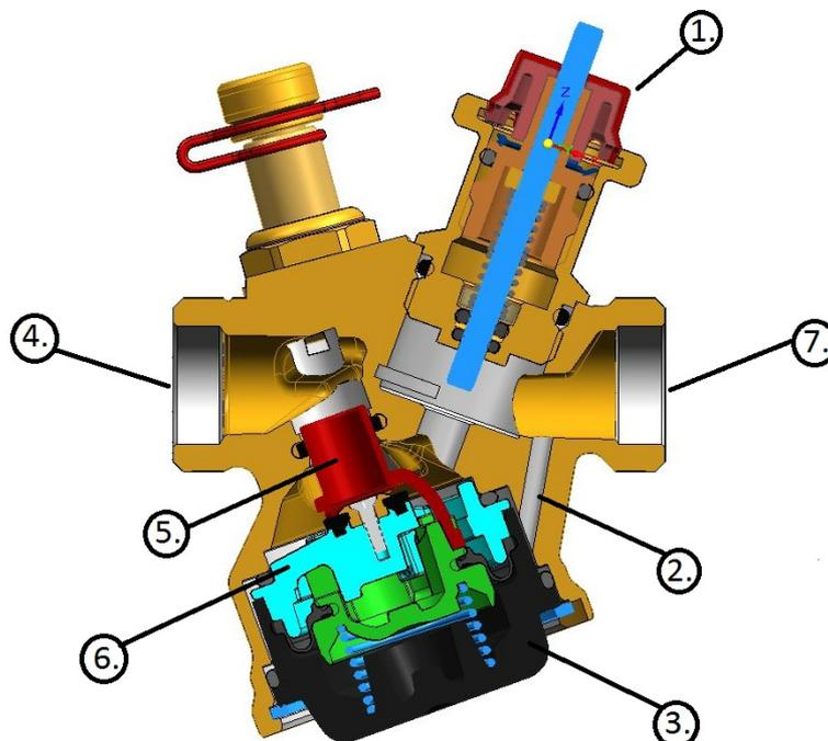
*Figure 4. A cross-sectional view on how the components operate in the product TA-Compact*
