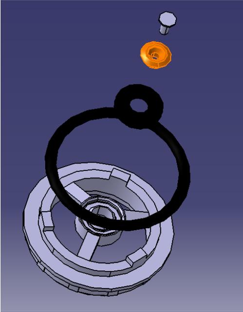
Figure 5. Exploding view on all the valve seat parts created in Catia V5.
