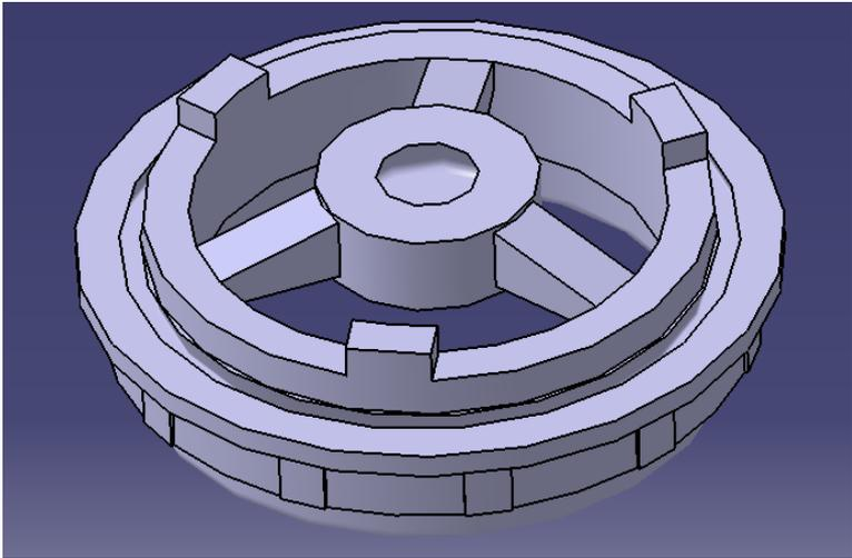
Figure 12. Upper view of concept three created in Catia V5
