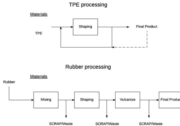
Figure 1. The differences between TPE and rubber processing. Adapted with permission from Hexpol TPE
