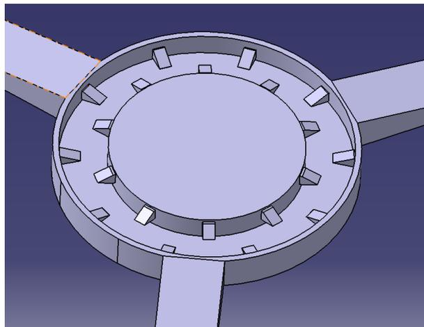
*Figure 6. A Catia V5 model for the initial idea for concept 1's mechanical lock*
