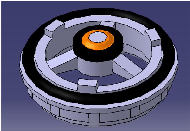
Figure 6. A visualization on the existing valve seat product created in Catia V5
