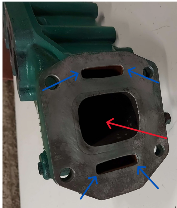
Figure 2.8: End of manifold where turbo attaches. (Blue=coolant channels. Red=exhaust gas channel)
