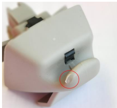
Figure 12. Picture of the defects identified on the sun visor hook.
