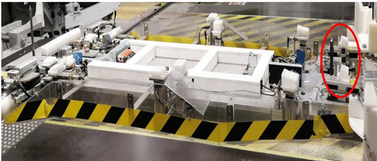
Figure 28. Picture of the V90 palette, the contact lugs to the support bearing are the white fixtures in the red circle.
