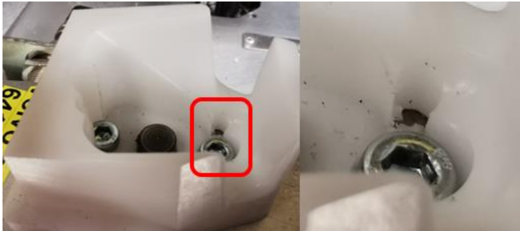
Figure 31. Picture showing defects in the contact lug.
