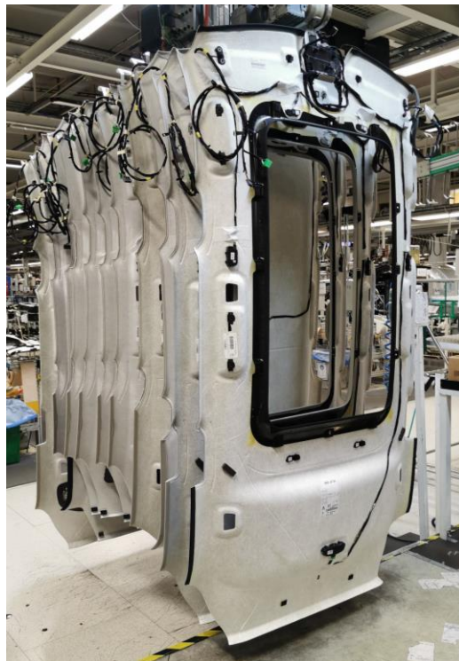
Figure 14. Picture of the headliner before it is put onto the palette and attached to the car body.
