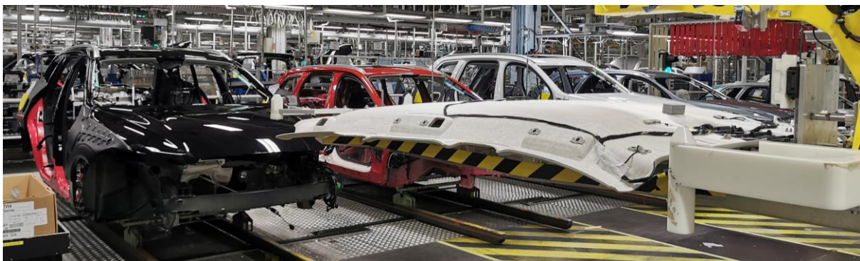
Figure 17. Picture of one headliner placed on a pallette ready to be moved into the car and attached to the car body.
