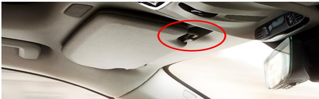
Figure 1. Picture of the sun visor and placement of the support bearing (Volvo Cars, 2020b).
