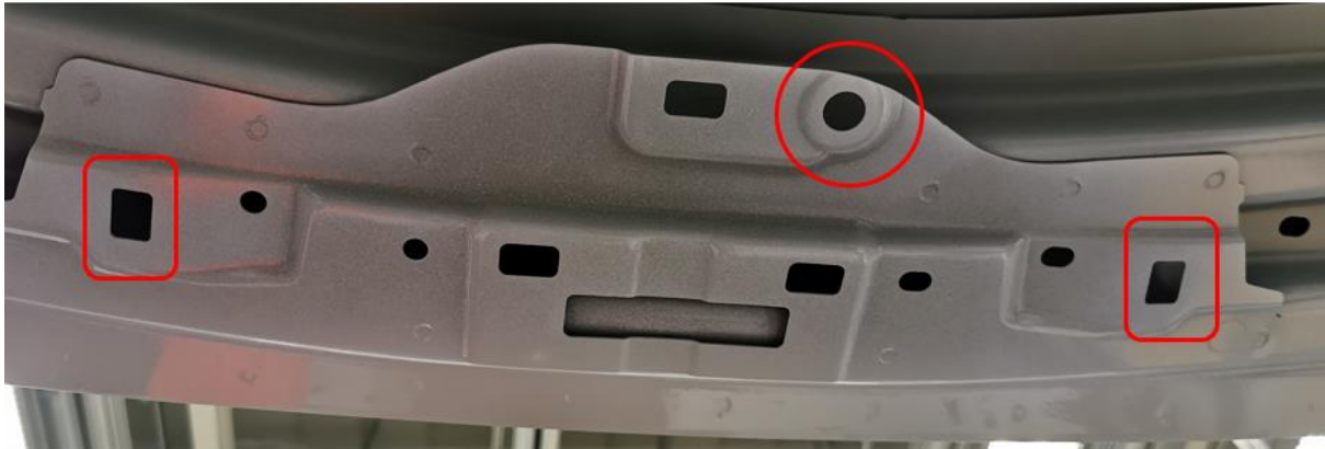
Figure 13. A picture on one of the consoles to the V90 where the support bearings attach. The two holes marked by red squares are where the support bearing attaches and the hole in the red circle is one positioning hole.
