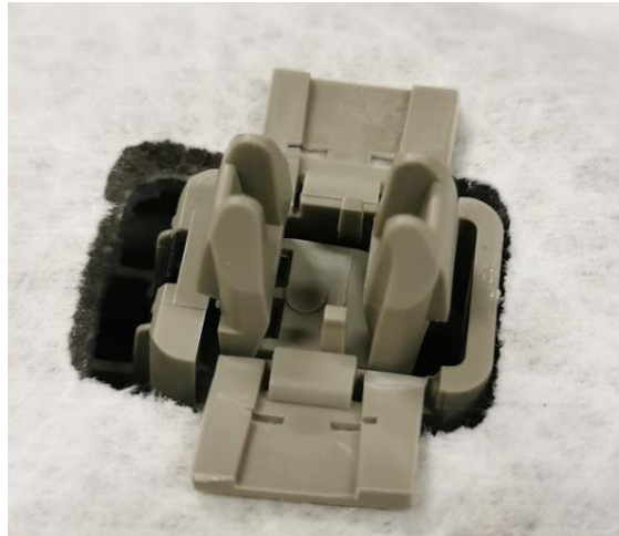
Figure 15. Showing the placement of the support bearing to the headliner, it is attached by the transport clips to make sure it does not fall off during the transportation between the stations.
