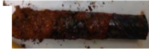
Figure 2. Rebar sample after corrosion.
