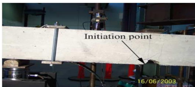
Fig: 8 Debonding of FRP strip[4]
