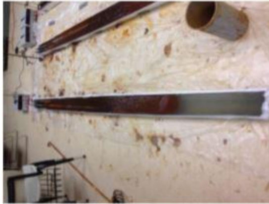
Figure 6. Steel rebars are corroding during the test.
