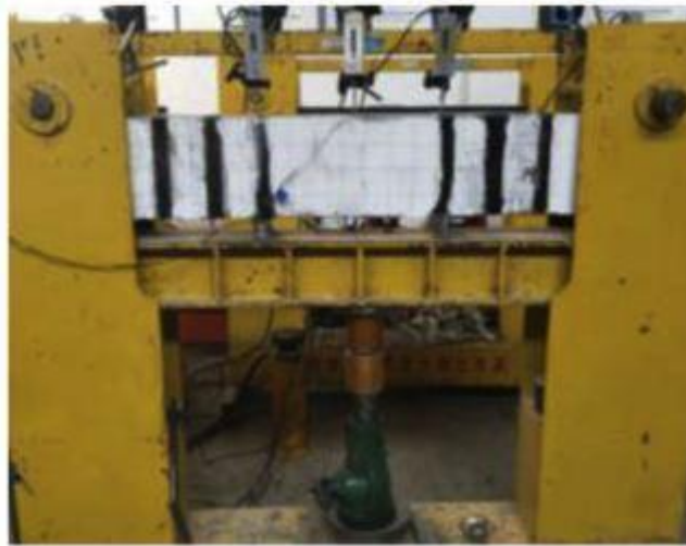
Fig: 21 Experimental test for CFRP strengthened beam - ref(19)
