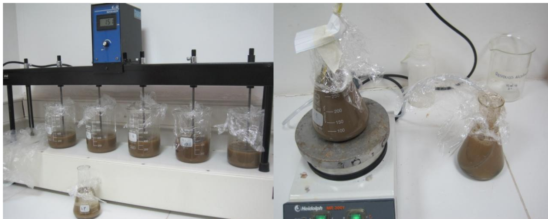
Figure 2. Ongoing process of a batch test. Left: There is a multispindle stirrer mixing sediment and river water. Right: Hotplate with a magnetic stirrer and a beaker with air injection.
