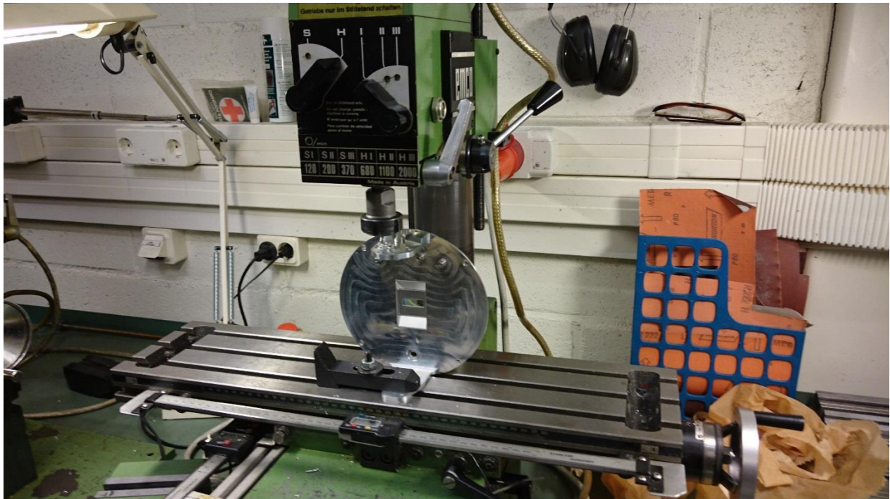
Figure 5.2: Drilling a hole pattern for the new motors.
