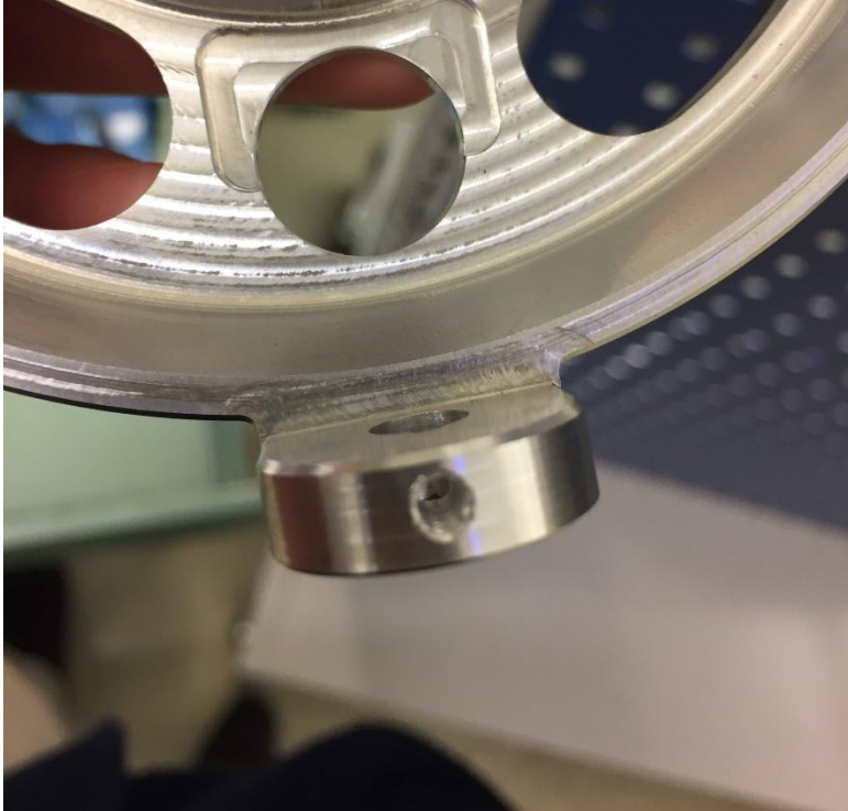
Figure 5.4: Threaded hole for a set screw securing the motor shaft.
