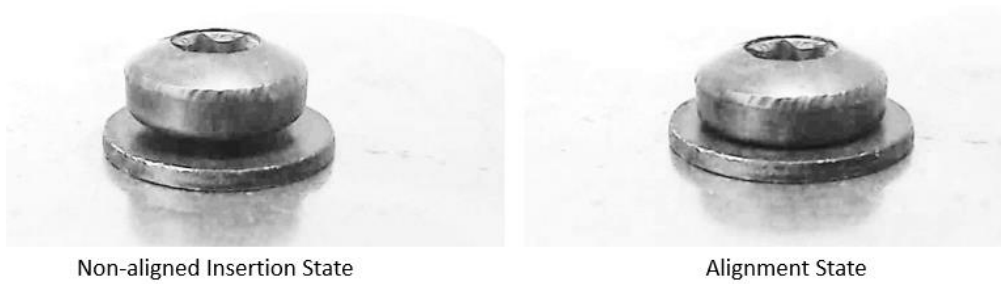
Figure 12. A visualisation of Insertion state and Alignment state while mounting a screw
