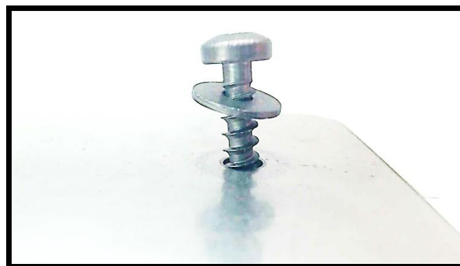
Appendix A Figure 5. Test 9 where a screw was inserted into a plate
