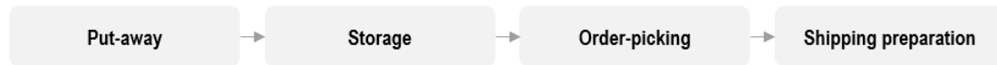
Figure 2.2: Visualization of the four warehouse processes (Kusrini et al., 2018; Brewer et al., 2001; van Gils et al., 2018), restructured from Kusrini et al. (2018). The four processes visualized facilitate the warehouse activity and include put-away storage, order-picking, and shipping preparation.
