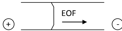
Fig. 2.2, of a EOF flow inside the capillary where the wall is negatively (-) charged, fixed layer is cover by the positive (+) ions and the diffuse layer containing a mixture of (+) (-) and neutral (n), move forward the negative end.
