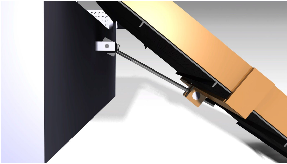
Figure 36 show the mechanical design concept of how to change the angle of the transporter.
