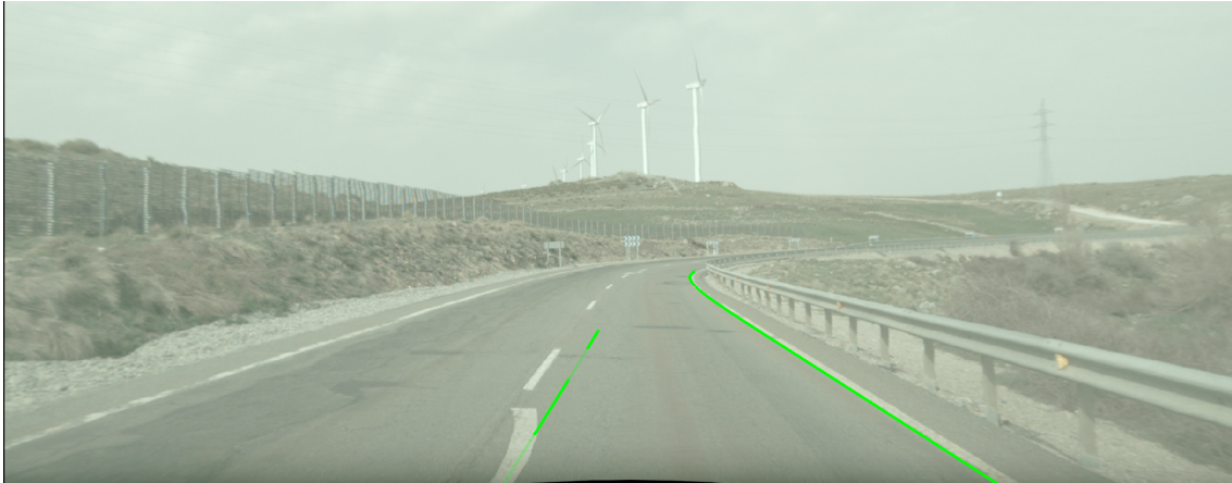
Figure 2.1: Sample instance of a false positive: the system identified the left lane marker to be closer than it actually is
