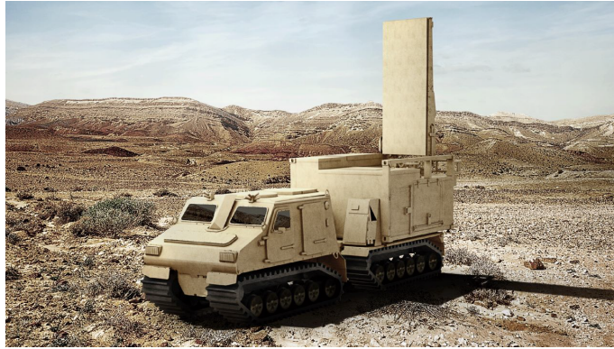
Figure 2.1: An ARTHUR unit mounted on a track-based vehicle where the radar system’s shelter can be observed on the rear part, hitched to the pulling bandwagon.[1]
