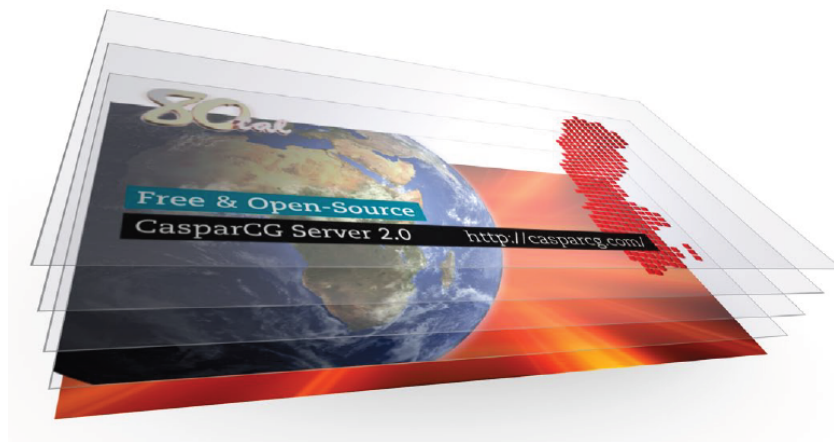
Figure 5.3: The output is composed of multiple video layers in CasparCG .
