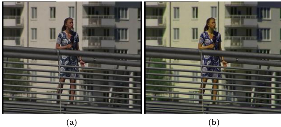
Figure 6.2: The tinting error where the output (b) has a yellowish tint 1 in relation to the reference in (a).
