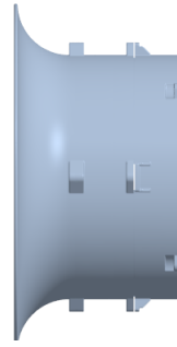
(d) Case D: Fan with shroud, cylindrical duct, and bell-mouth
