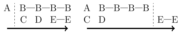
Figure 2.6: Execution graphs which show available parallelism for two different solutions, with B and E having real costs of 4 and 2 respectively. It is clear that the left graph is a better solution because it represents a more parallel evaluation.
