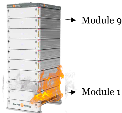
Figure 50 Corvus Energy Rack with 9 Modules TR Initiated (Module 1)
