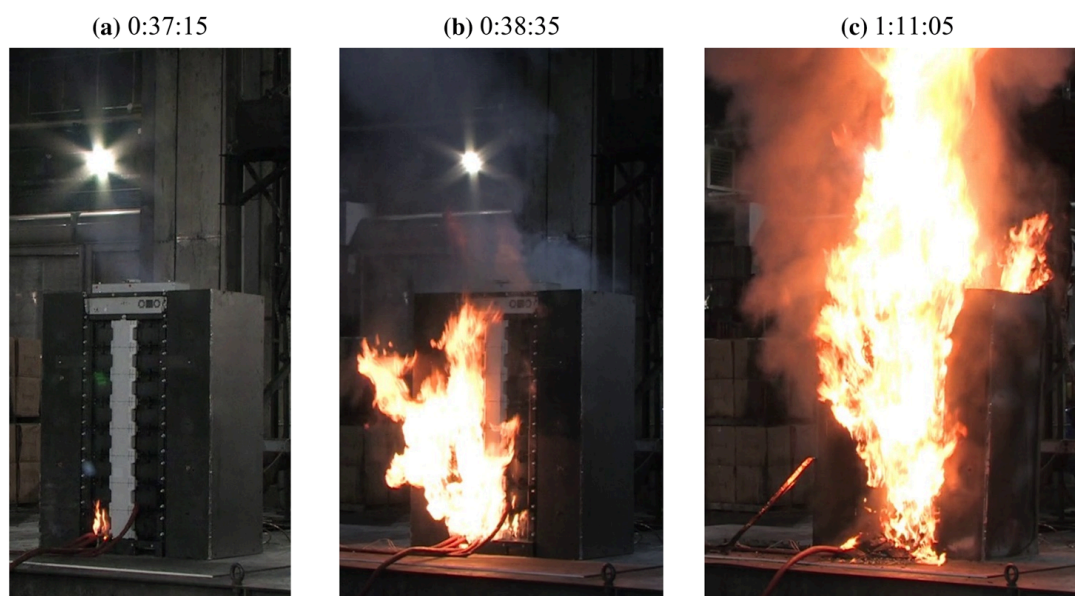
Figure 23 LFP fire development during large-scale (16 Modules) 83kWh free burn test: near time of ignition (a), near time of predicted sprinkler[4]
