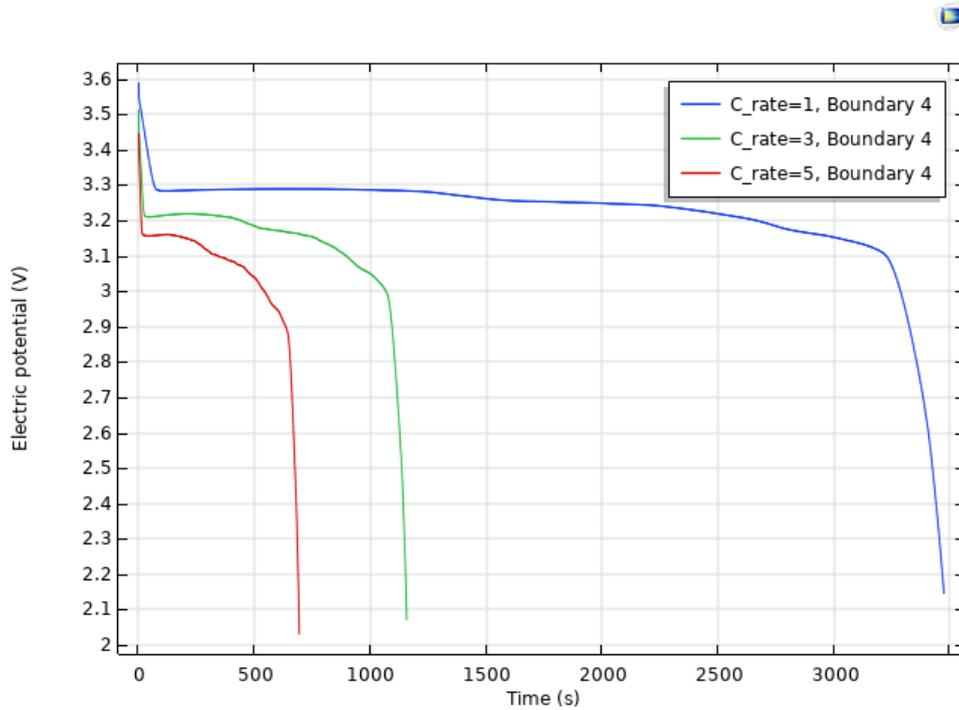
**Figure 4.2:** Potential curve of the structural cell under different current rates
