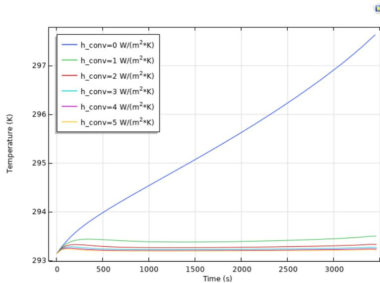
**Figure 4.6:** Temperature profile at 1C discharge current under different convection
