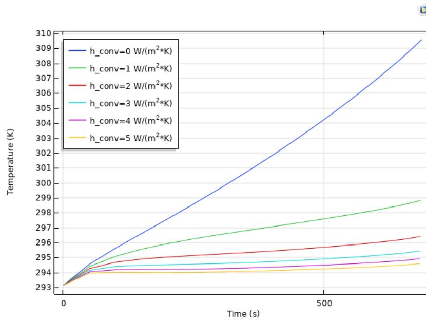
**Figure 4.8:** Temperature profile at 5C discharge current under different convection
