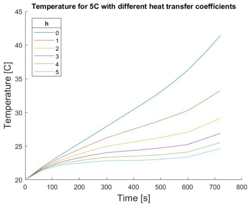
**Figure 4.12:** 5C temperature profile under convection conditions, from [3]
