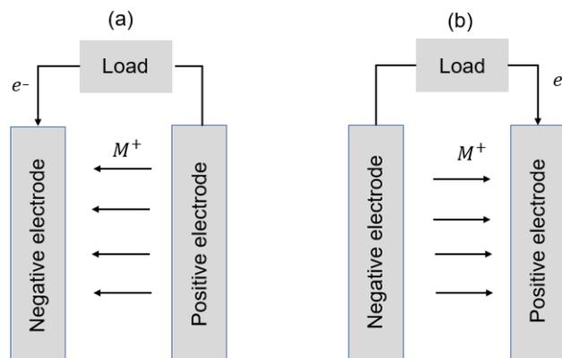
**Figure 2.1:** (a) An electrolytic cell (b) a galvanic cell (both retrieved from [4])
