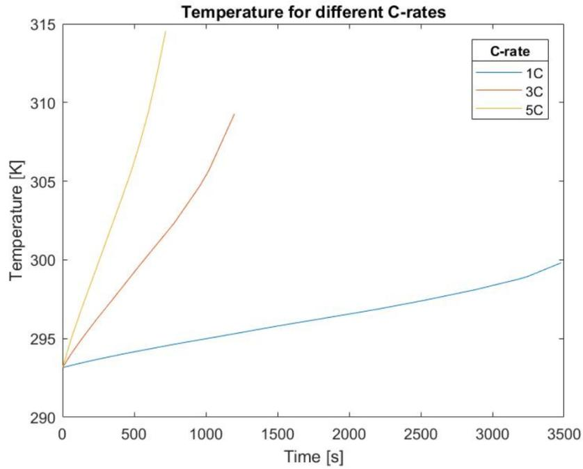
**Figure 4.9:** Temperature profile at different C rates without natural convection, from [3]
