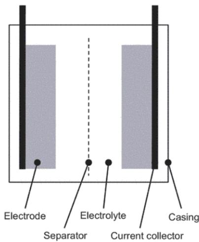
**Figure 2.2:** The fundamental design of an electrochemical cell from [4]
