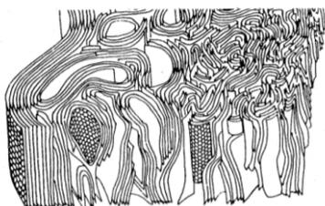
**Figure 2.3:** Carbon fiber internal structure from [5]
