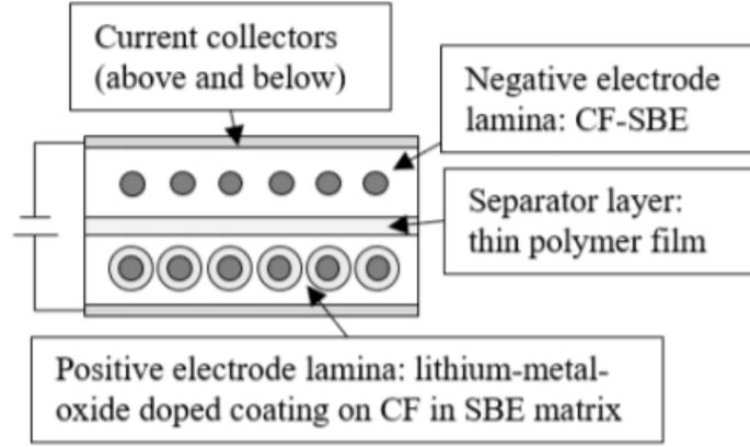
**Figure 2.4:** Schematic illustration of the laminated structural battery composite architecture, retrieved from [11]
