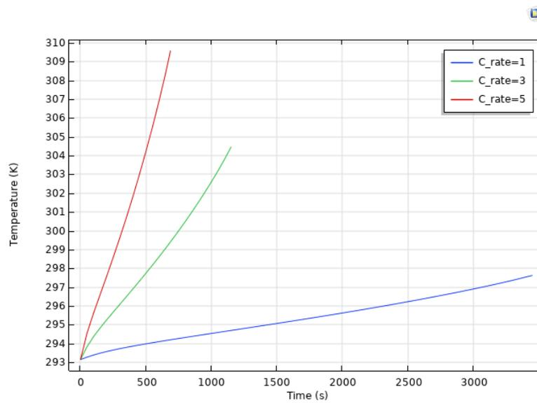
**Figure 4.5:** Cell temperature under different current rates, captured at boundary 1
