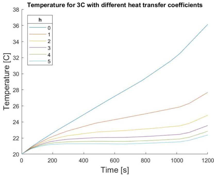
**Figure 4.11:** 3C temperature profile under convection conditions, from [3]
