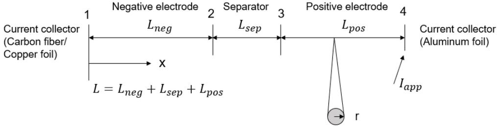
**Figure 2.5:** Schematic of P2D model: 1D (x-direction) structural cell coupled with microscopic (r-direction) particles
