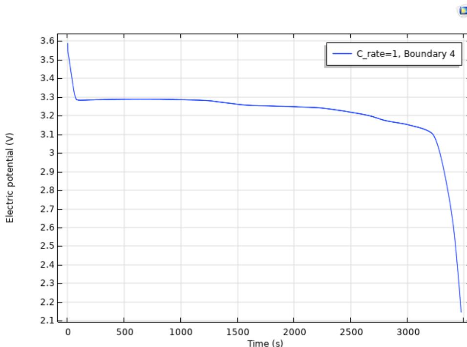
**Figure 4.1:** Potential curve of the structural battery cell at 1C
