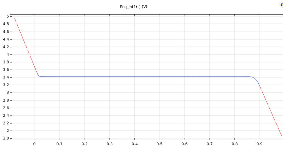
**Figure 3.2:** Equilibrium potential for LFP as function of SOC
