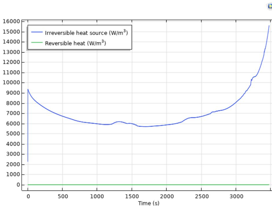
**Figure 4.3:** Thermal contributions of the structural cell at 1C discharge
