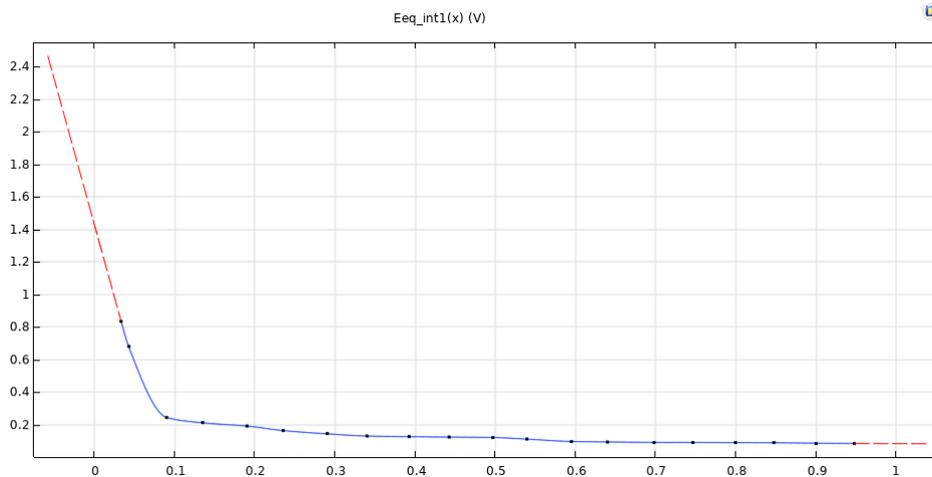
**Figure 3.1:** Equilibrium potential for CF as function of SOC
