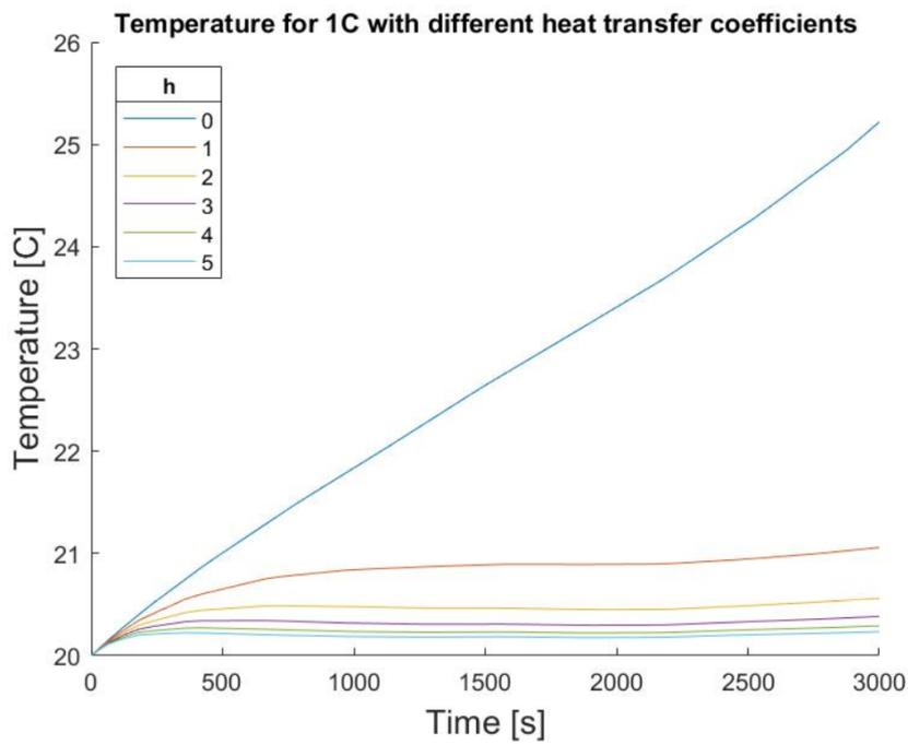
**Figure 4.10:** 1C temperature profile under convection conditions, from [3]
