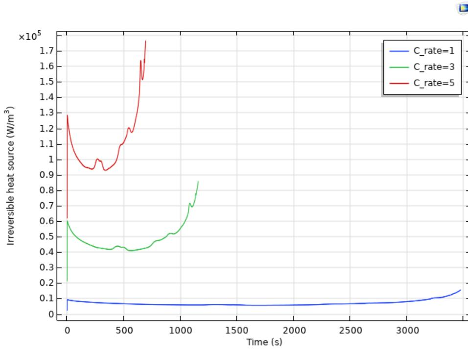
**Figure 4.4:** Power dissipation at different current rates
