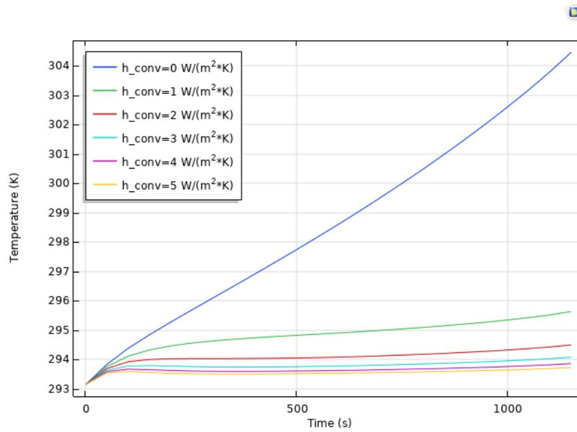
**Figure 4.7:** Temperature profile at 3C discharge current under different convection
