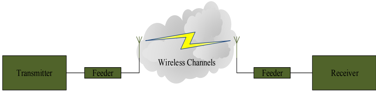
Figure 3.1: A block diagram of a wireless communication system
