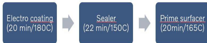
Figure 6: Image of the different curing temperatures and times for the test samples.
