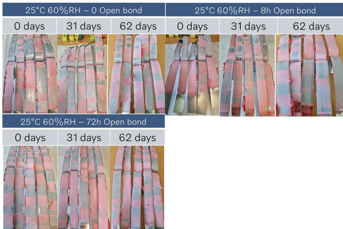
Figure 12: How open time/closed time and ageing days influences the peeling strength and failure mode. In all scenario appearances of cohesive and surface near cohesive failure can be indicate.
