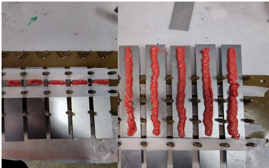
Figure 5: Image of the how the specimen with certain amount of open time are placed in their respectively climate condition. Left corresponds to lap-shear samples while right is T-peel specimens.
