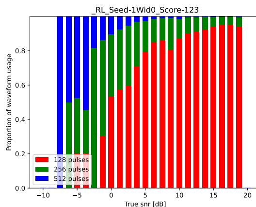
Figure 4.9: Number of pulses used when tracking targets with SNR shown on the x-axis. The SNR values are estimated SNR for 128 pulses of integration.
