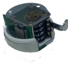
Figure 4.2: A mechanical counter with a BLE chip
