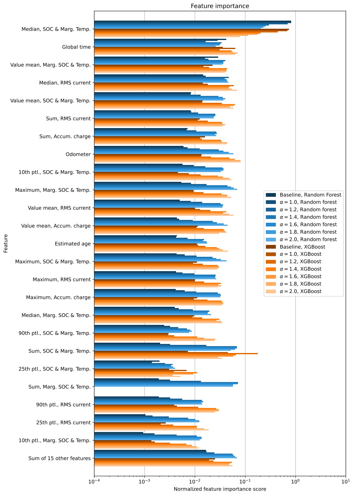
Figure 5.9: The feature importance scores computed for the weighted models trained on the Vehicle Fleet Dataset using different \alpha values. Features for which all models have importance scores below 2 \cdot 10^{-2} are summed to improve readability.
