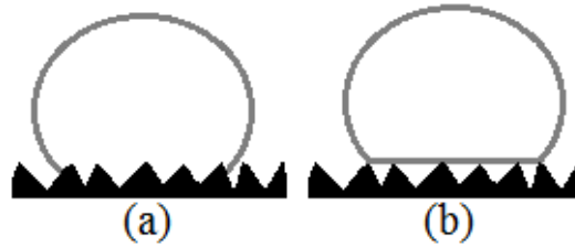
Figure 2.3: The different wetting models (a) Wenzel and (b) Cassie-Baxter (Yan et al. 2011).
