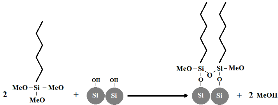
Figure 2.6: The dehydration reaction between the silanol groups of the silica and a silane.
