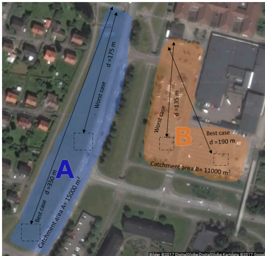
Figure 5.4: Worst and best case excavations, longest flowing distance d marked (Google, 2017). Published in accordance with Google copyright policy.
