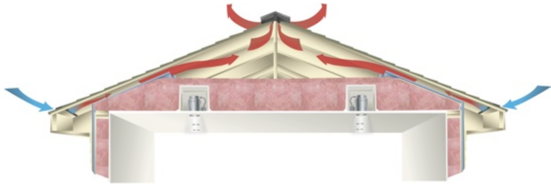
Figure 1.1: A ventilated cold attic seen from the side [3].
