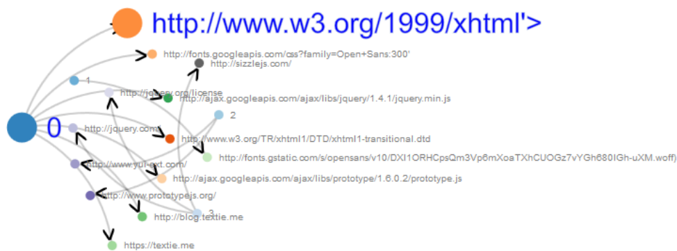
Figure 5.3: The directed edge showing the linking between ID 0 and the URL http://www.w3.org/1999/xhtml
