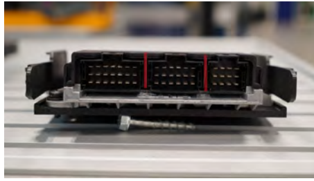
Figure 4.8: Tolerances between Sockets(red marked)
