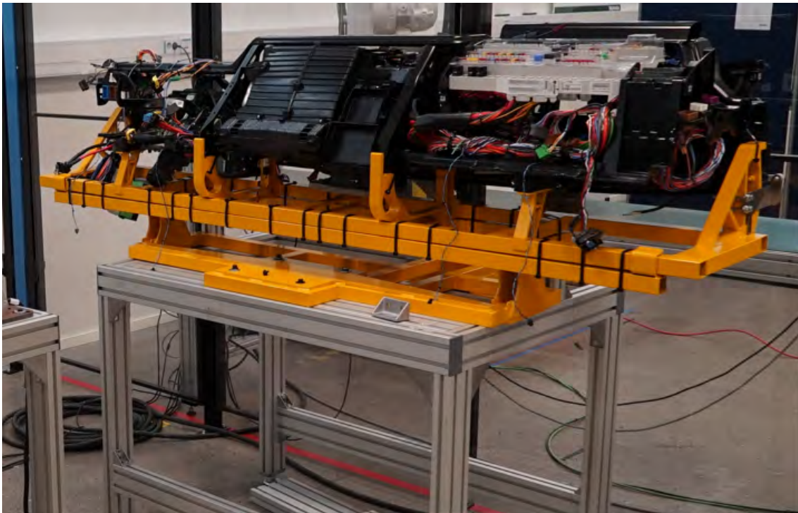
Figure 4.2: Test Setup of Instrument Panel in the Smart Factory Lab
