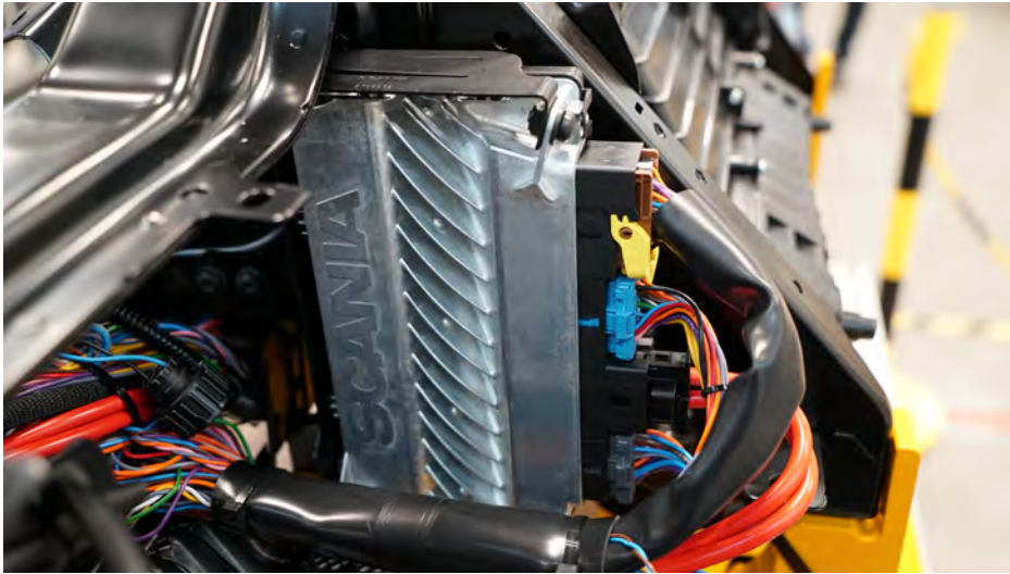
Figure 3.2: ECU assembled to the instrument panel with 4 connected cables
