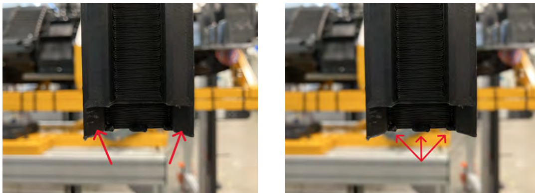
(a) Chamfered Edges(red arrows)
