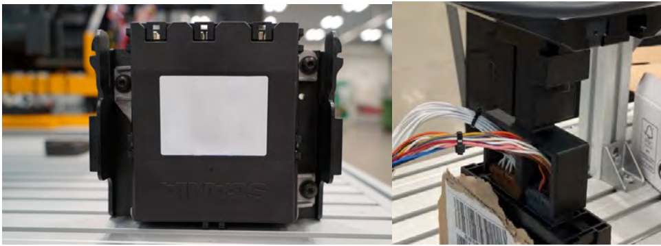
(a) ECU with Three Sockets(Side View) (b) Joining Tool for Two Connectors
