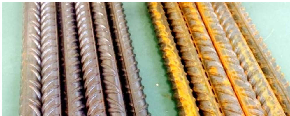
Figure 21 Reinforcement bars before and after being manually brushed
