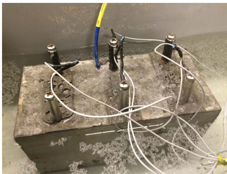
Figure 22 Beam partially subjected in a 10%NaCl solution
