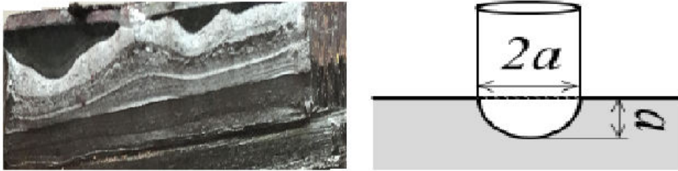
Figure 7: Comparison between real fatigue crack ( black zone) and artificially created crack shapes
