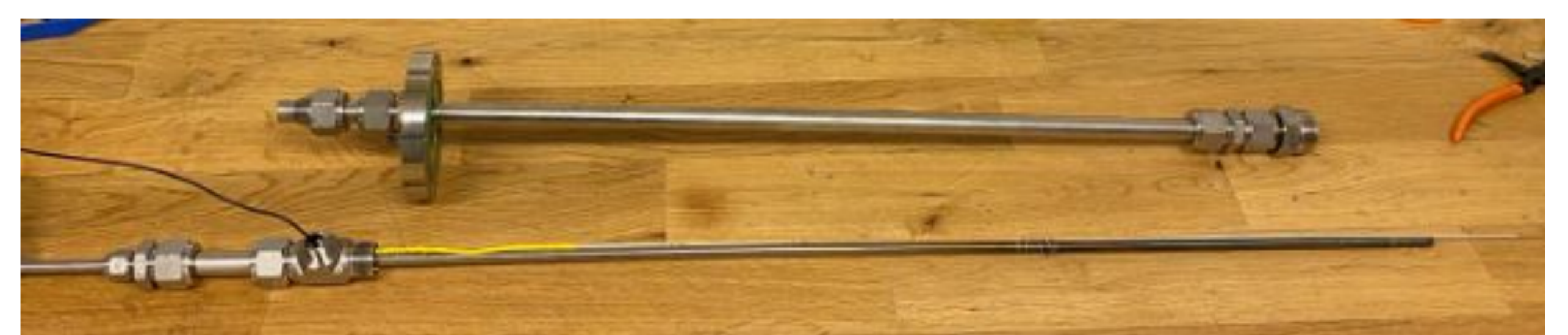
Fig: Outer tube and inner tube with the platinum wire attached to it.
