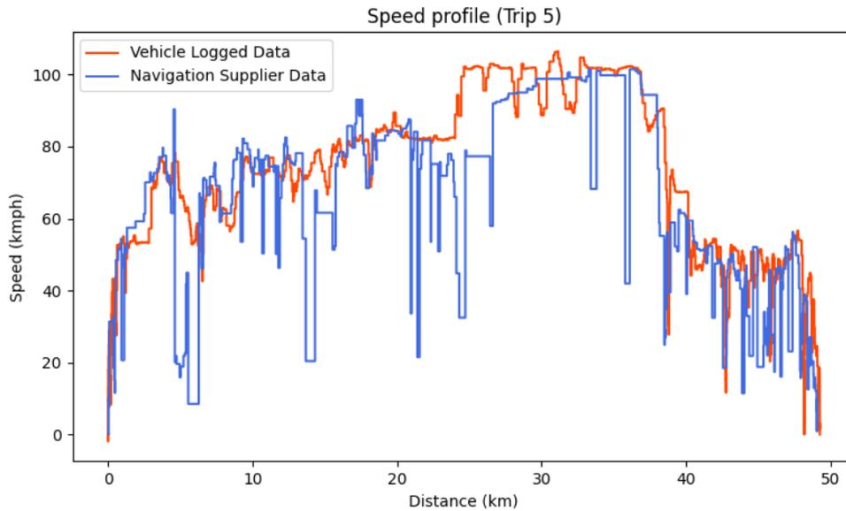
**Figure 4.7:** Speed profile for trip 5 from both navigation supplier data and vehicle logged data
