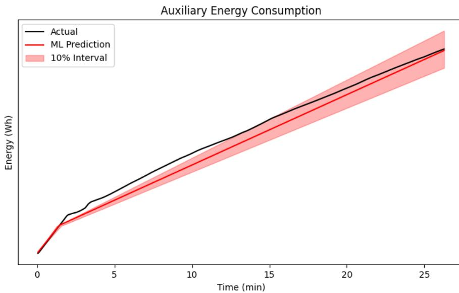
**Figure 4.21:** Auxiliary energy consumption prediction interval for trip 1 obtained from mixed-XGB model on vehicle logged data for 10% speed variation.
