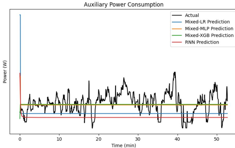
**Figure 4.18:** Auxiliary power predictions for trip 6 from all the auxiliary ML models. Due to slightly warmer day and preheated compartment, the transient phase is negligible.
