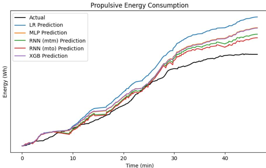
**Figure 4.8:** Propulsive energy consumption predictions for trip 5 obtained from all the propulsive ML models on navigation supplier data.
