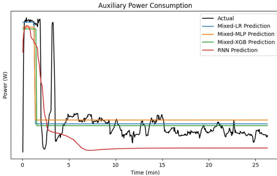
**Figure 4.15:** Auxiliary power predictions for trip 1 obtained from all the models on vehicle logged data. The trip was taken on a colder day and hence the transient phase is pronounced.
