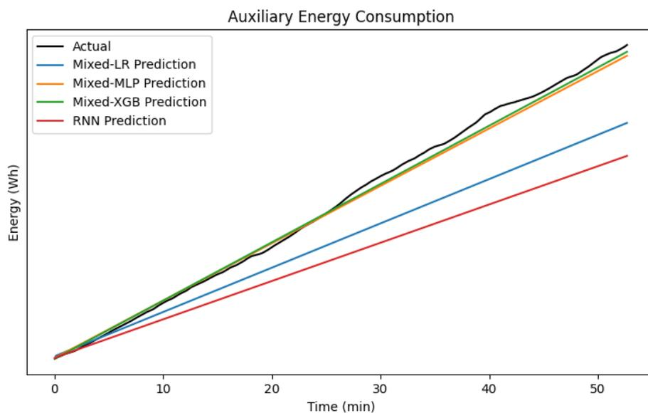
**Figure 4.19:** Auxiliary energy predictions for trip 6 from all the auxiliary ML models. The predictions have almost a constant slope throughout the trip as transient phase is negligible.
