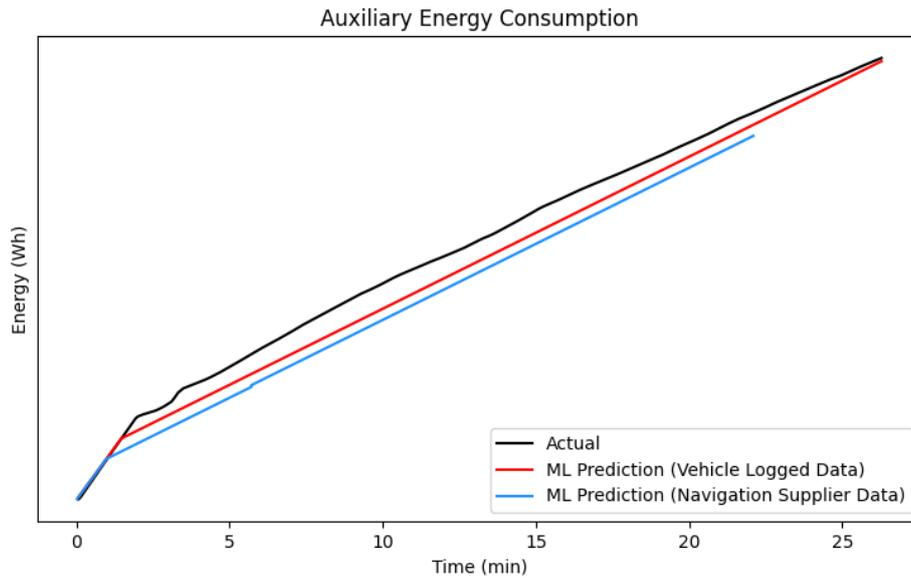
**Figure 4.14:** Auxiliary energy predictions for trip 1 obtained from mixed model with gradient boosting on both navigation supplier and vehicle logged data.
