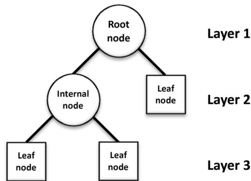
**Figure 2.4:** Schematic for a single decision tree [17].
