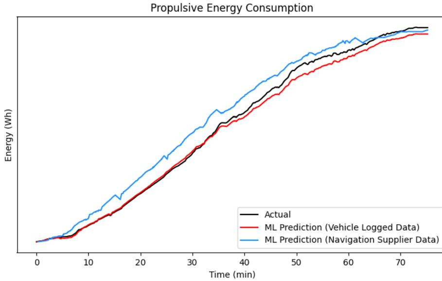
**Figure 4.5:** Propulsive energy consumption for trip 2. The graph shows actual consumption value and predictions on both navigation supplier data and vehicle logged data obtained by RNN many-to-many model.
