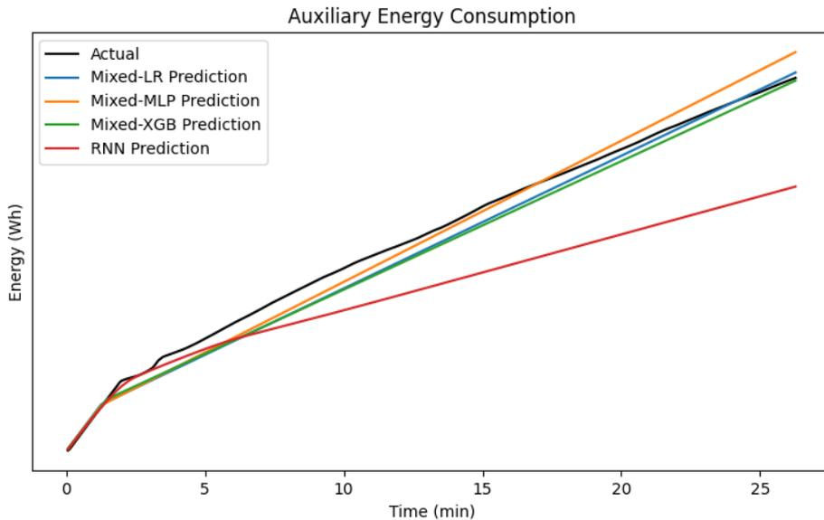
**Figure 4.16:** Auxiliary energy consumption predictions for trip 1 obtained from all the models on vehicle logged data. Predictions from different models except RNN are very close to each other and the actual consumption.
