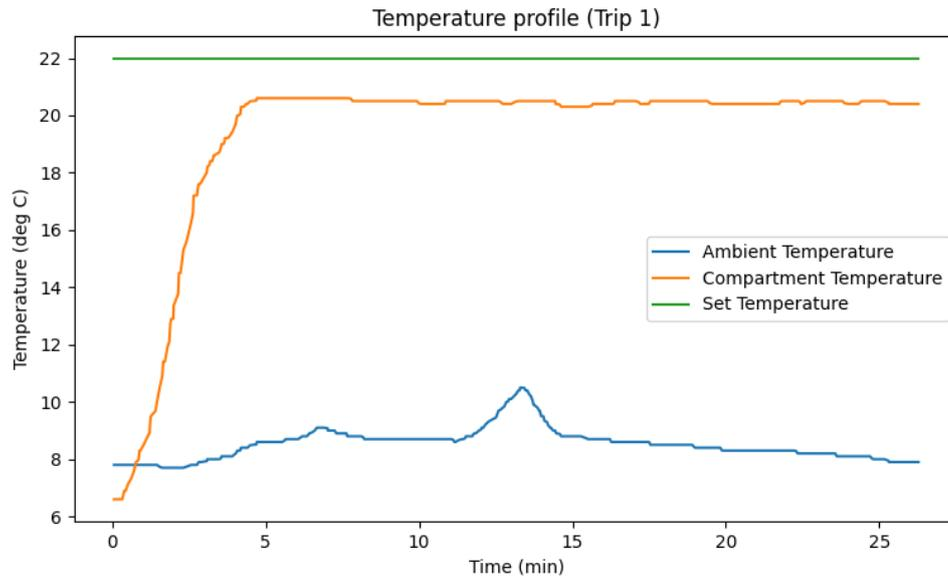
**Figure 4.12:** Temperature profile for trip 1 from vehicle logged data.
