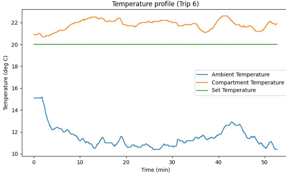
**Figure 4.17:** Temperature profile for trip 6 from vehicle logged data.
