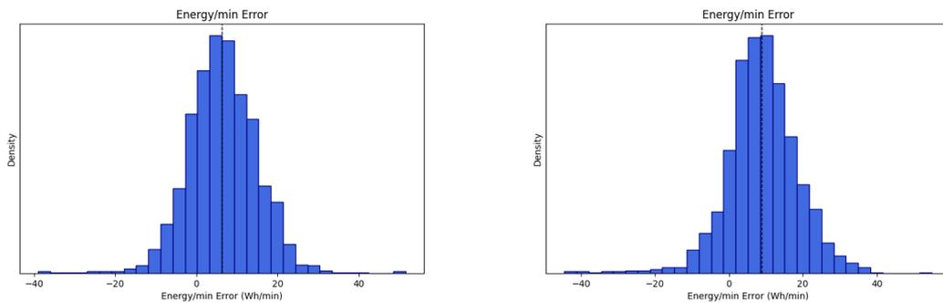
(a) Histogram for Mix-XGB model errors with median value of 6.28 (b) Histogram for RNN model errors with median value of 8.80
