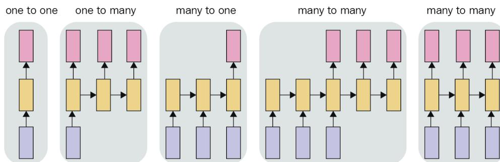
Figure 2.3: Different types of RNN architectures [15]
