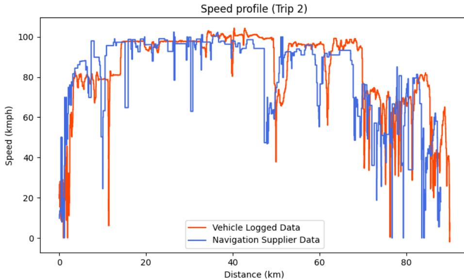
**Figure 4.4:** Speed profile for trip 2 from both navigation supplier data and vehicle logged data
