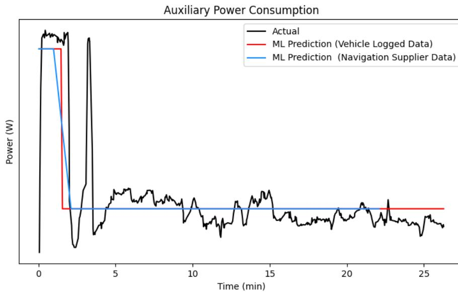
**Figure 4.13:** Auxiliary power predictions for trip 1 obtained from mixed model with gradient boosting. The model is able to predict the duration and power level of transient phase reasonably well.
