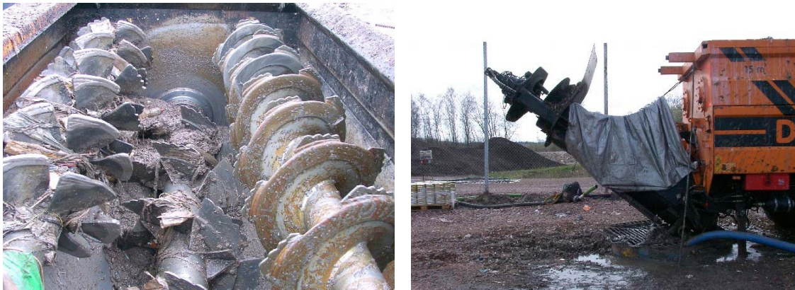
Figure 4.2 Mixing chamber with mills and screw shaft in the bottom followed with screw press.
