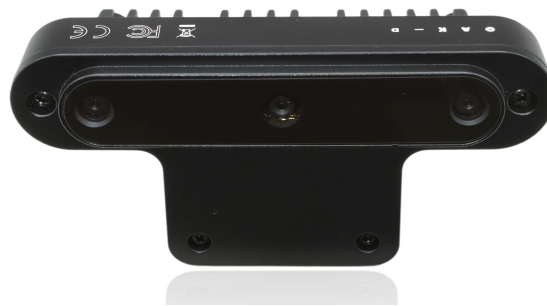
Figure 4.7: Luxonis OAK-D stereoscopic camera with built-in IMU. Image source:[51]
