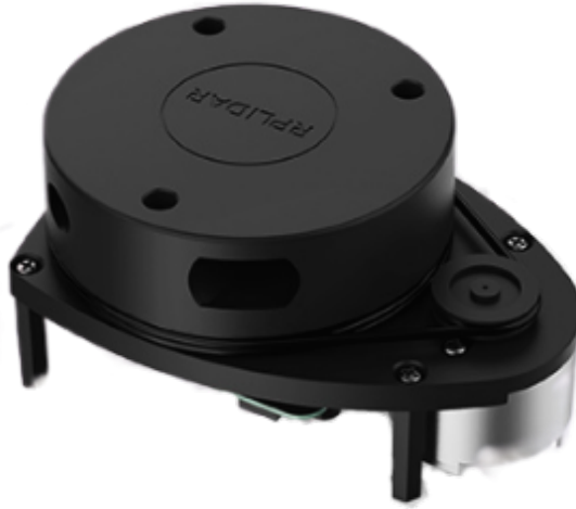
Figure 4.5: Slamtec RP LIDAR A1. Image source:[50]
