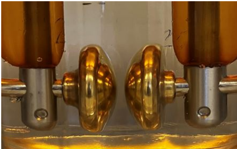
Figure 4.3: AC Breakdown testing electrode setup
