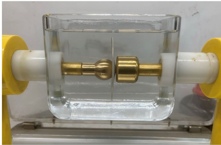
Figure 4.5: AC Breakdown testing for the material
