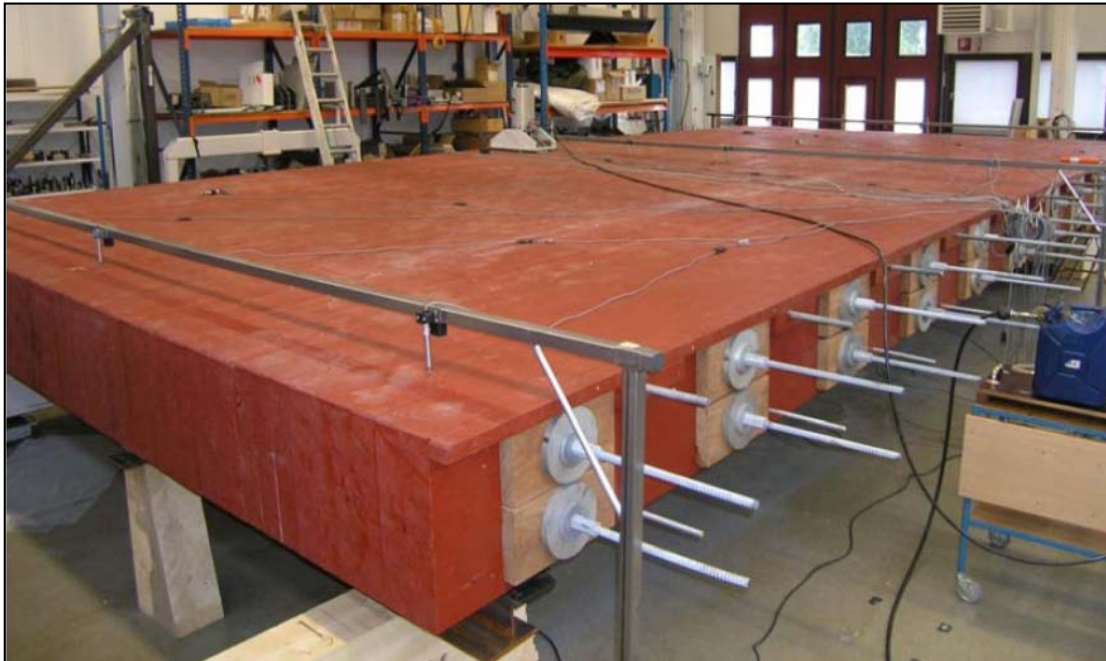
Picture 2.1 Test of full scale bridge. Force plate mounted at edge in mid-span, top-centre of picture (Courtesy of Martinsons Träbroar).
