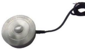
*Figure 3.6: FC23 compression load cell*
