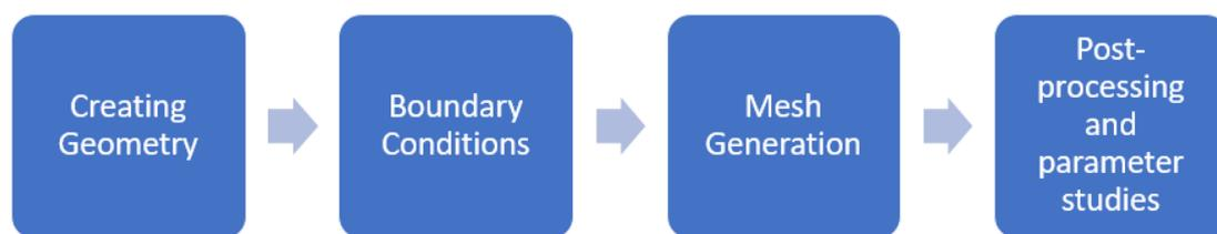
*Figure 3.13: Steps of the simulation methodology*
