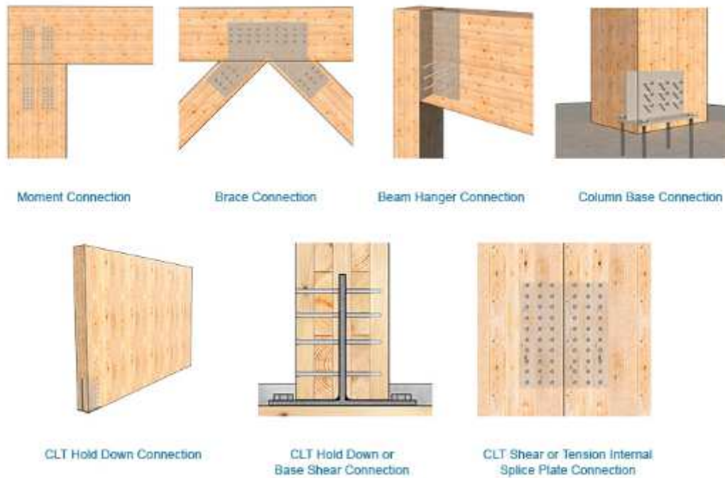
Figure 2.8 Dry connections in timber structures
