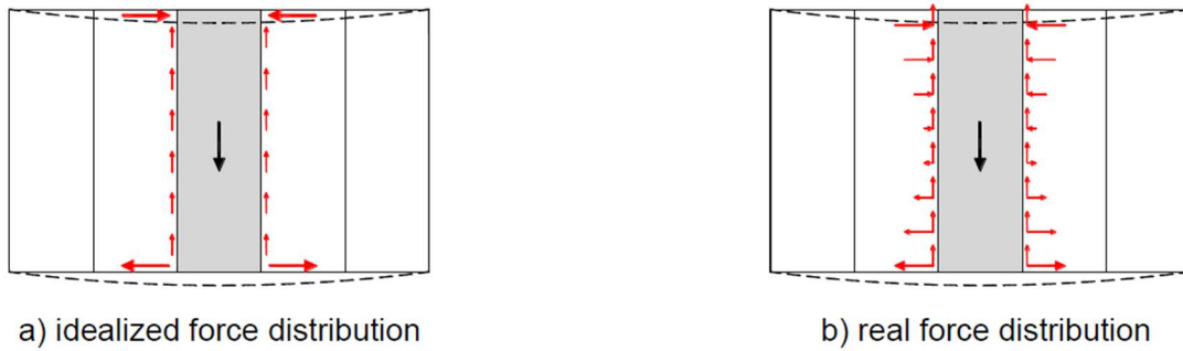
a) idealized force distribution b) real force distribution Figure 4.10 Force distribution for diaphragm panel connections subjected to deep beam behavior.
