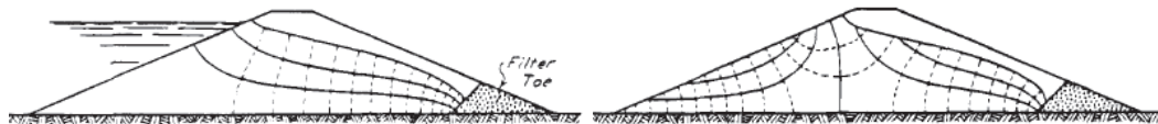
Figure 8 Different scenarios illustrating change in flow net due to rapid loss of resisting load (Terzaghi et al., 1996).
