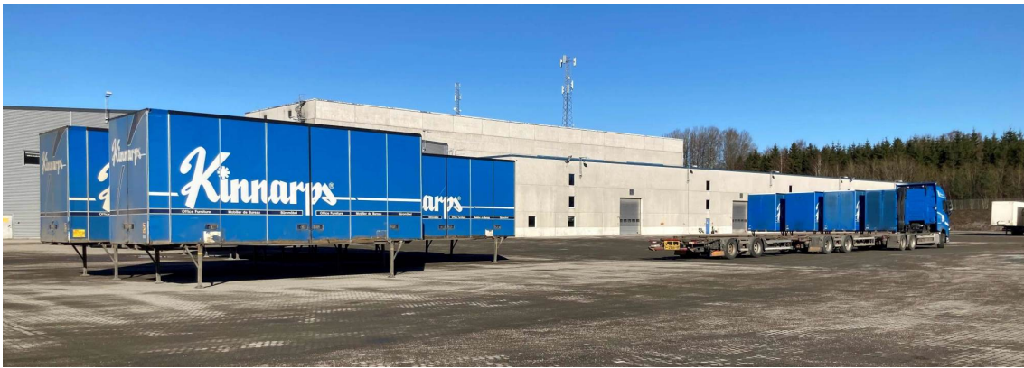
Figure 3.10: A DUO-CAT combination to the right reversing towards a swap body to later fasten it on the trailer, in an open area.
