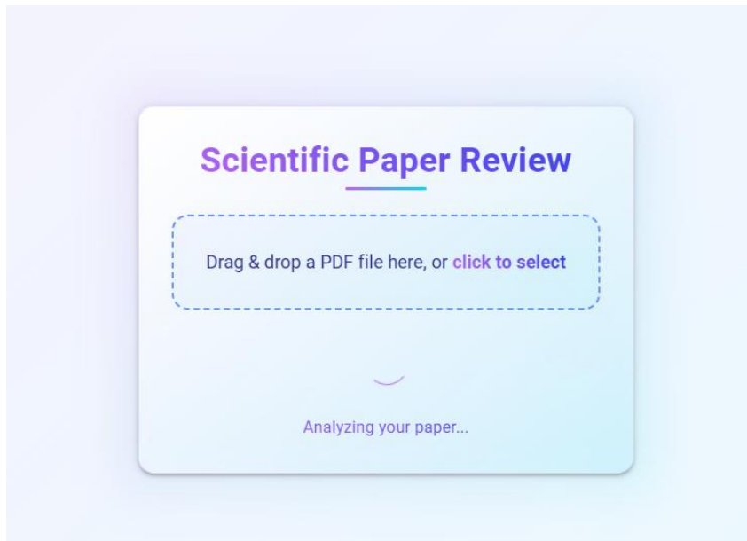
Figure 2: Closer view of the FileUpload-component. It consists of a container at the middle with a dropzone which allows users to select their pdf-file by either dropping it in or by selecting it locally. In this figure, a file has already been selected for review and the app is processing it, as can be seen with the “Analyzing your paper” status text.
