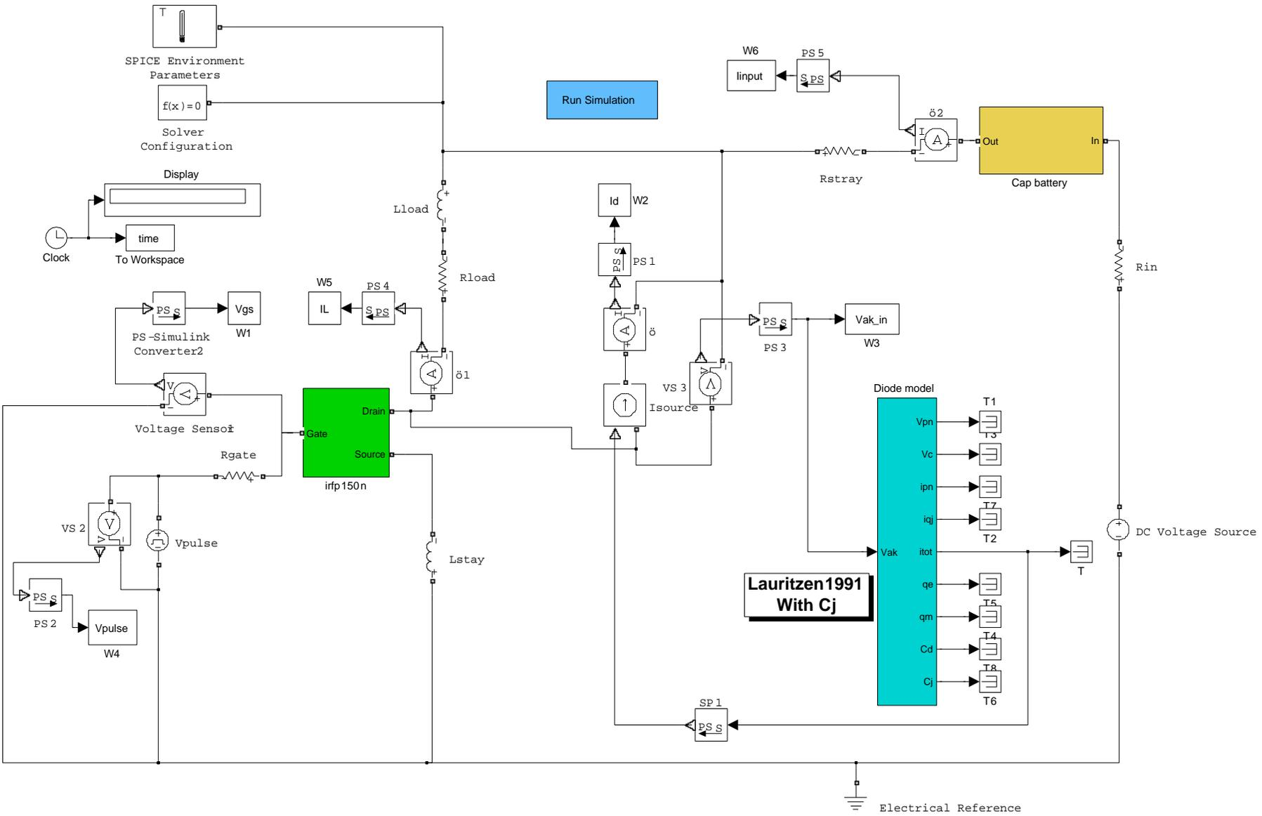
Figure F.4 – Diode tester circuit implemented in SimElectronics.
