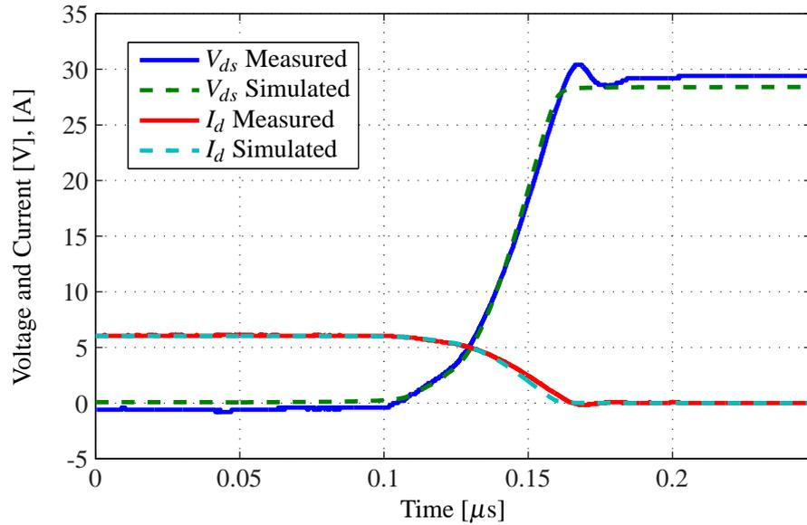
**Figure 5.7** – The turn-off transition from both measurement and simulation. The simulation result is gathered from a model where all parasitic and stray components are omitted.
