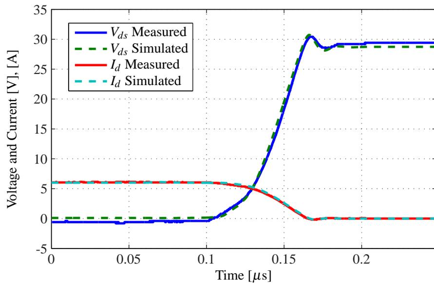
**Figure 5.8** – The turn-off transition from both measurement and simulation. The simulation result is gathered from a model where parasitic and stray components are accounted for.
