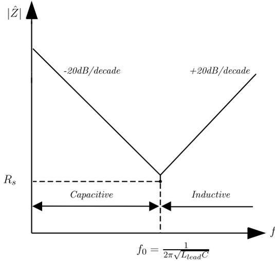
2.5.b: The impedance of the nonideal capacitor plotted against frequency.
