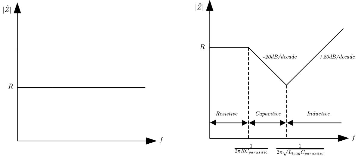
2.3.a: The impedance of the ideal resistor plotted against frequency.
