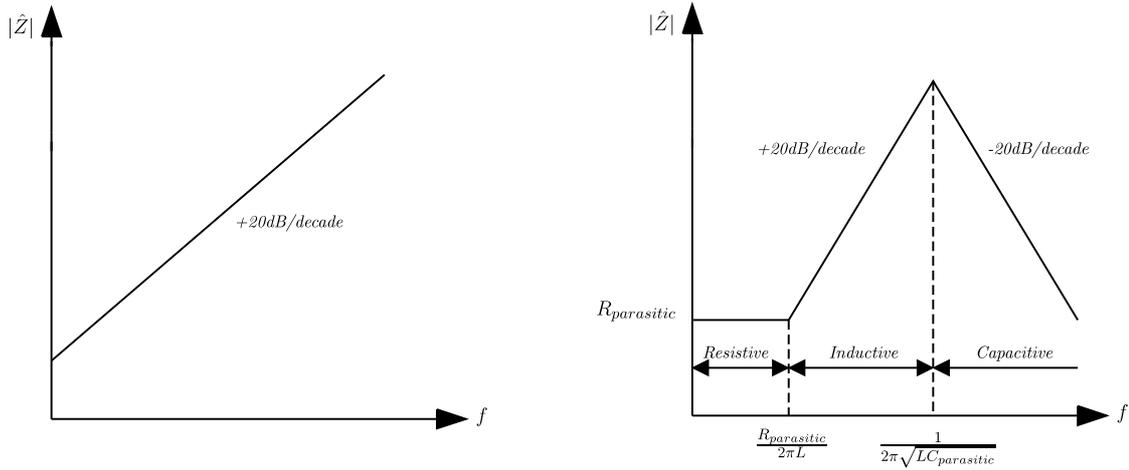
2.7.a: The impedance of the ideal inductor plotted against frequency.
