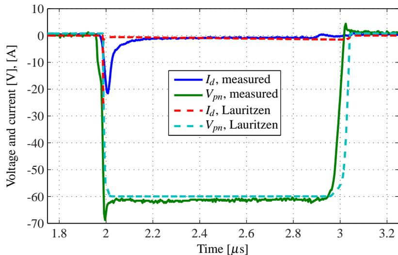
**Figure 6.5** – Measured and simulated drain current and diode voltage. The diode used during simulation is the implementation of the Lauritzen diode model.
