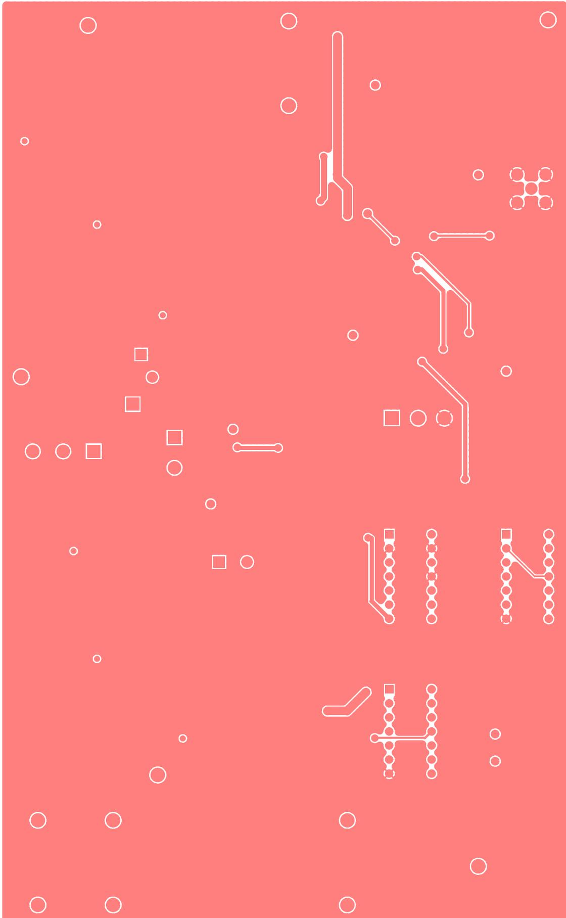
**Figure E.3** – Bottom PCB layer of the buck converter.
