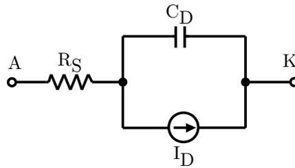
Figure 4.1 – Diode model.
