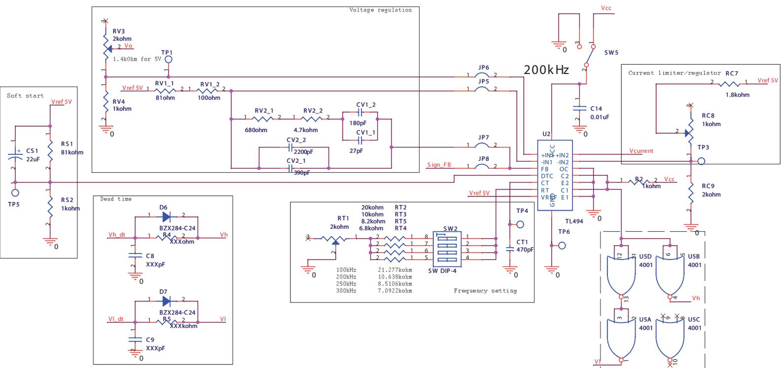
**Figure D.2** – Buck converter SPICE schematic designed in order to utilise the PCB layout software OrCad Layout. Sub-schematic 2 of 3.
