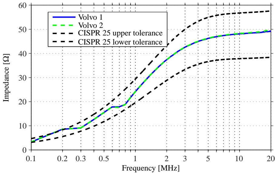
Figure 3.4 – Results from measurements on the LISN available at Volvo Cars AB.
