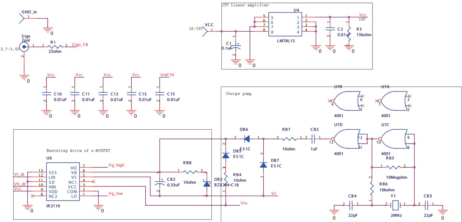
Figure D.3 – Buck converter SPICE schematic designed in order to utilise the PCB layout software OrCad Layout. Sub-schematic 3 of 3.
