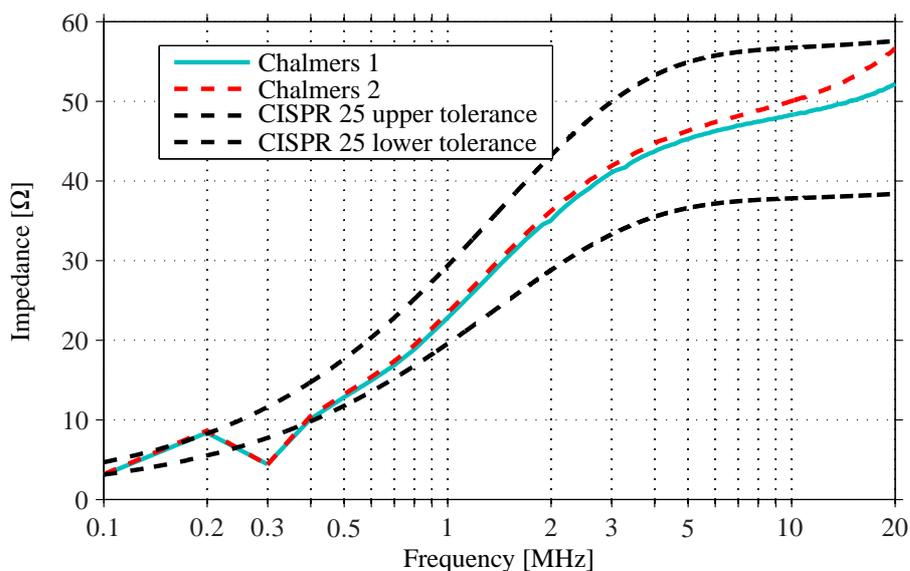
Figure 3.3 – Results from measurements on the self constructed LISN.
