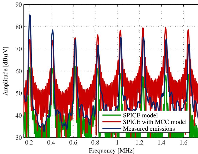
**Figure 6.10** – A comparison between measured frequency content and frequency content from simulations using both the conventional diode model and the MCC model.
