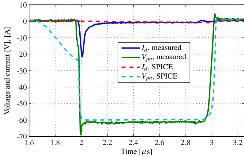
**Figure 6.4** – Measured and simulated drain current and diode voltage. The diode used during simulation is the conventional diode model supplied by the manufacturer.
