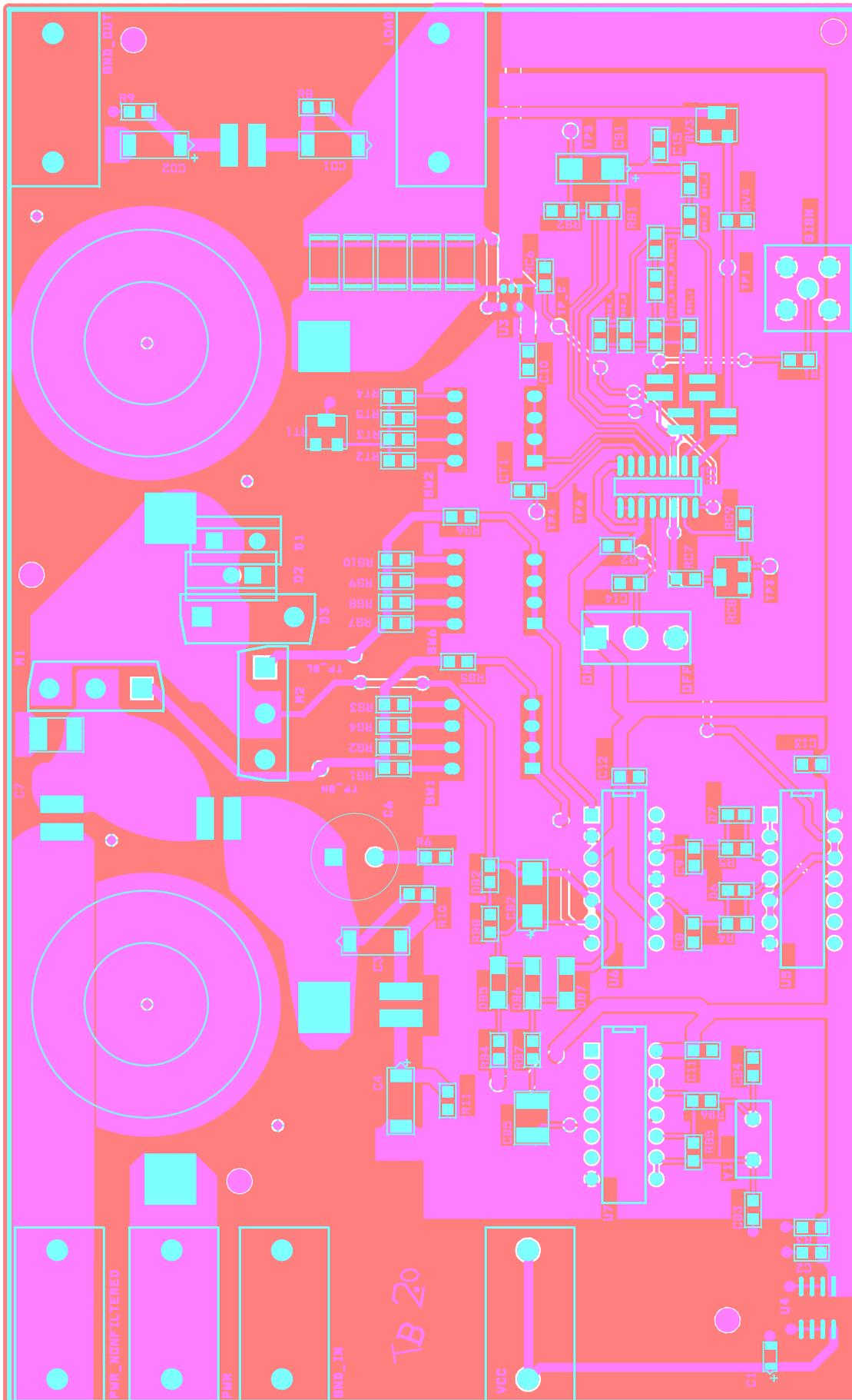
Figure E.4 – Component placement outlined over the PCB of the buck converter.
