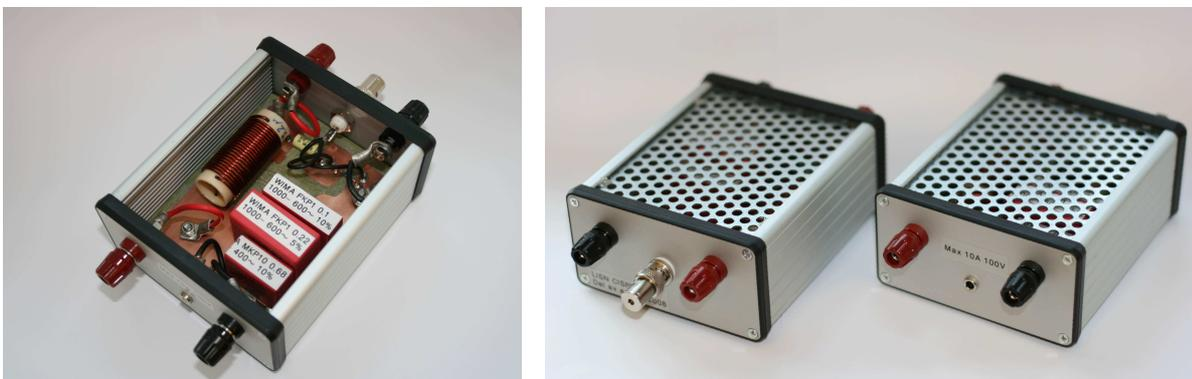
**Figure 3.2** – The inside of the finalized LISN and two LISN's in their casing.
