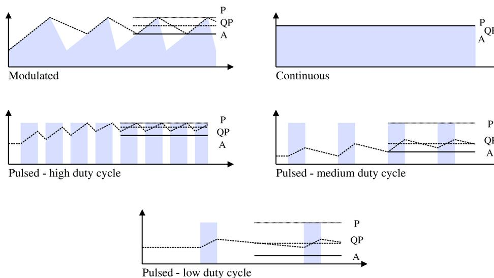
**Figure A.1** – Peak(P), quasi-peak(QP) and average(A) detectors indicating different levels of the same signal.
