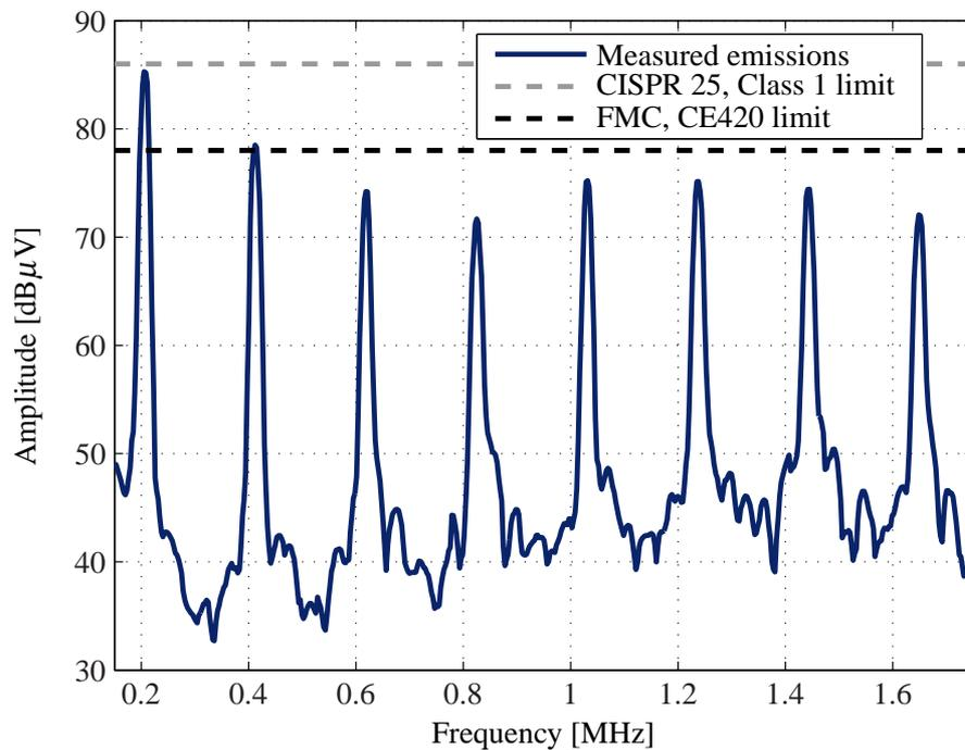
**Figure 6.8** – Measured frequency content in the MW band, conducted emissions.
