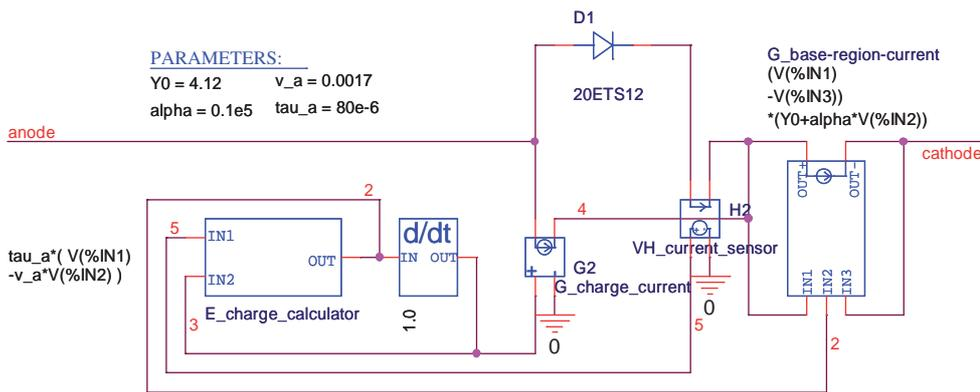
Figure 4.6 – Implementation of MCC in SPICE using ABM blocks.
