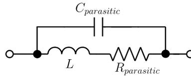
2.6.b: Nonideal inductor model with parasitic resistance and lead elements.
