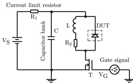
3.5.a: Simplified diode tester schematic.
