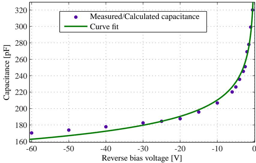
Figure 4.5 – Junction capacitance measured by utilizing a resonant circuit.
