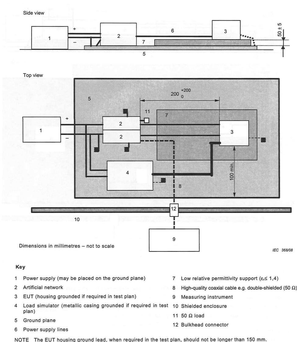
**Figure 2.1** – Measurement setup for measurement of conducted emissions, EUT with power return line remotely grounded. (Figure courtesy of IEC.)
