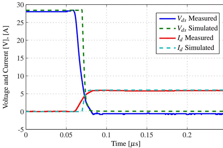
**Figure 5.5** – The turn-on transition from both measurement and simulation. The simulation result is gathered from a model where all parasitic and stray components are omitted.
