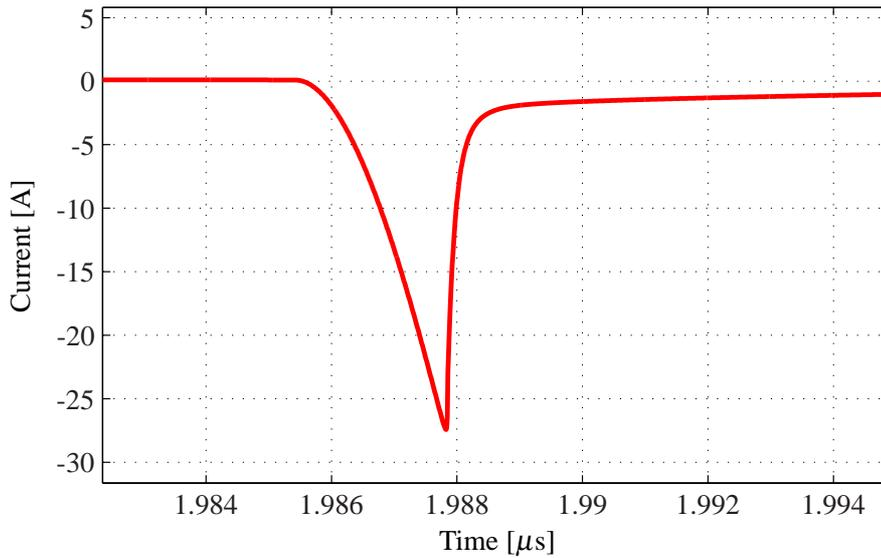
**Figure 6.6** – Simulation showing the MOSFET drain current. The model produces the correct reverse recovery shape although during a very short time.
