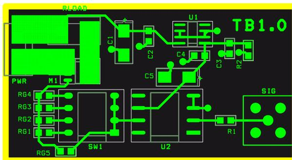
5.1.b: PCB layout of the test circuit created in OrCAD Layout.
