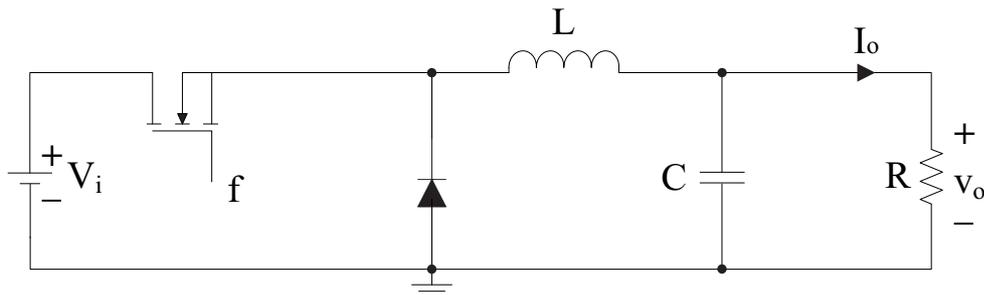
**Figure 6.1** – A basic buck converter.
