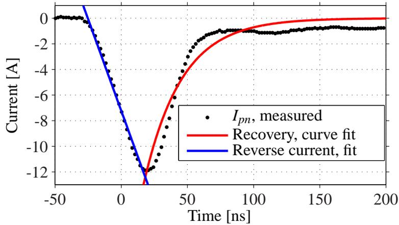
**Figure 4.3** – Reverse recovery waveform processed with the curve fitting toolbox in Matlab in order to extract required parameters.
