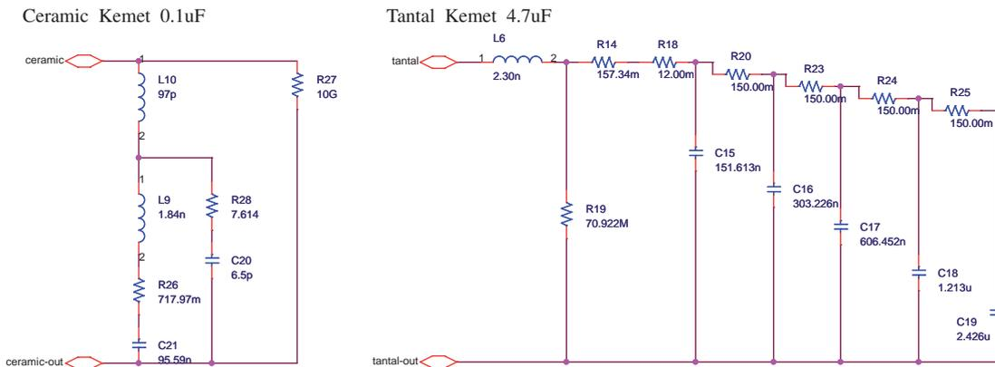
Figure 5.3 – Detailed capacitor model from Kemet.
