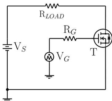
5.1.a: Basic switching circuit with a MOSFET in series with a load resistor.
