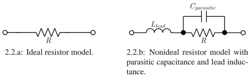
**Figure 2.2** – Ideal resistor (a) and a nonideal resistor (b).
