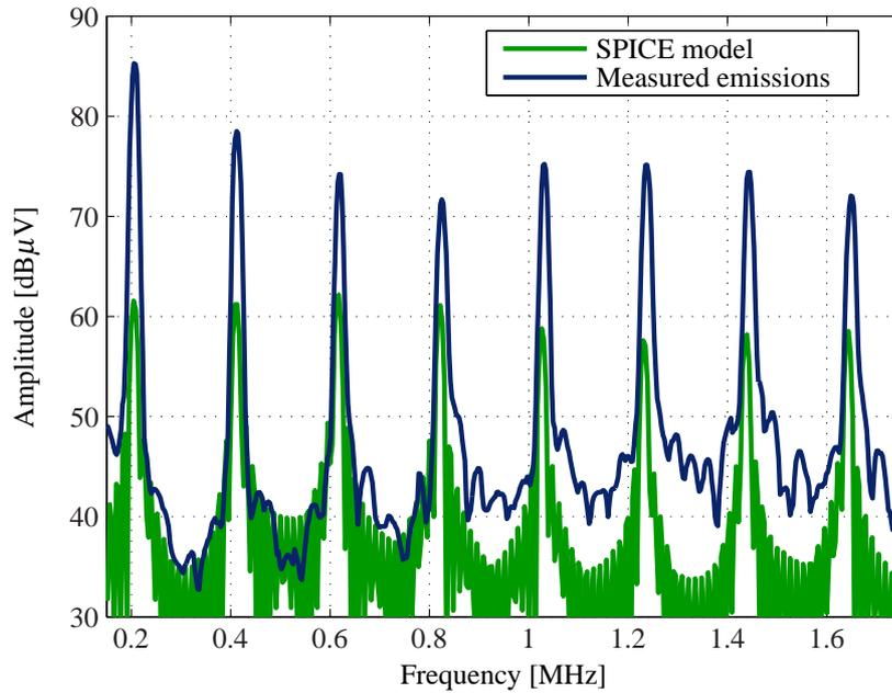
**Figure 6.9** – Frequency content from the simulated Buck converter using the conventional SPICE diode model from the supplier together with the measured frequency content.
