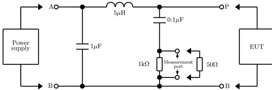
**Figure 3.1** – Schematic of a LISN or AN required for measurements according to the CISPR 25 standard. EUT refers to, just as DUT, to the device under test. (Figure courtesy of IEC.)
