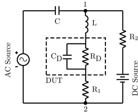
4.4.b: The diode is replaced by a capacitance in parallel with a resistor for analysis purpose.
