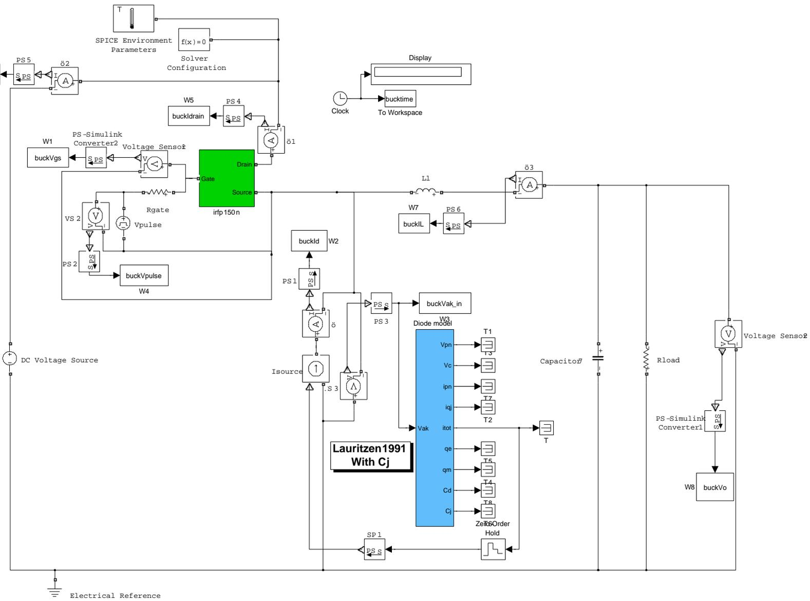
Figure F.3 – Buck converter implemented in SimElectronics with the Lauritzen diode model.
