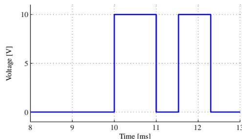
3.5.b: An example of a MOSFET gate voltage produced by the timer circuit.
