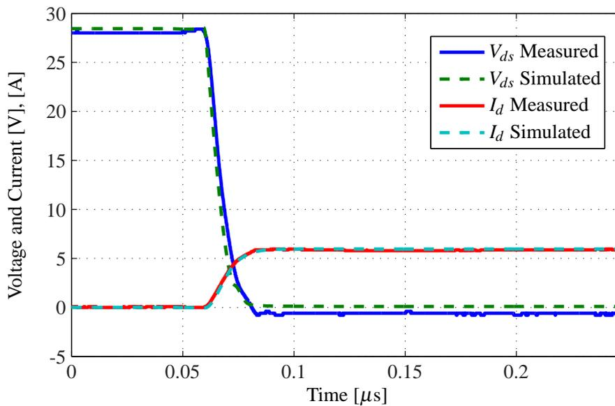
**Figure 5.6** – The turn-on transition from both measurement and simulation. The simulation result is gathered from a model where parasitic and stray components are accounted for.
