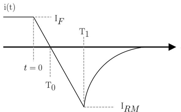
**Figure 4.2** – Diode turn-off current waveform used in the parameter extraction.
