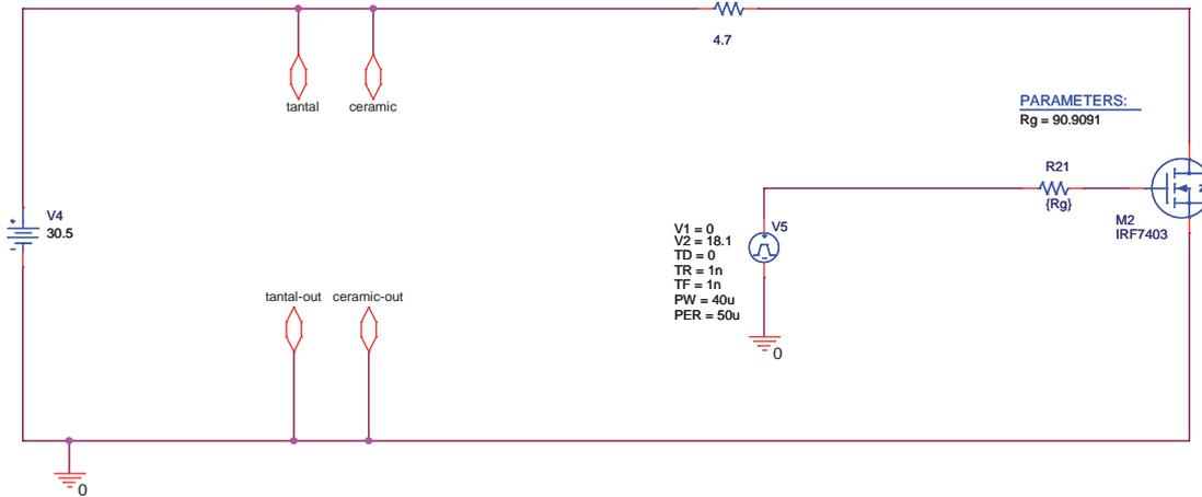
Figure 5.2 – Simple model of TB1.
