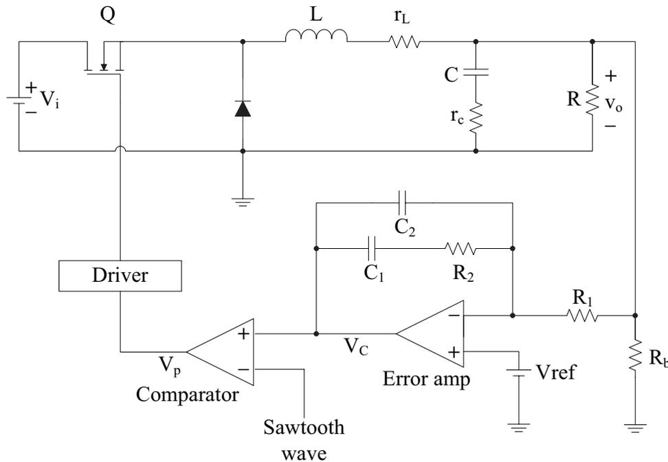
**Figure 6.2** – Buck converter with voltage control loop.
