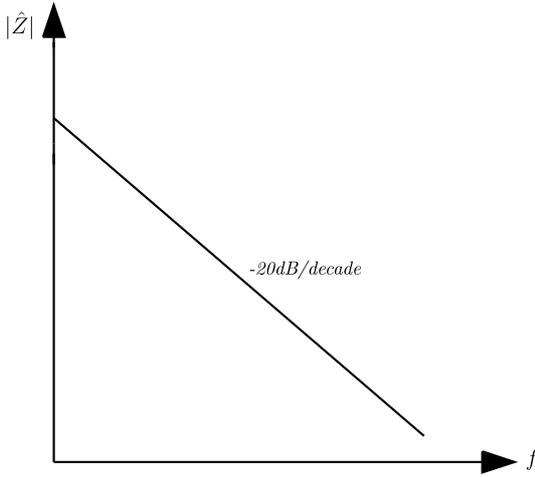
2.5.a: The impedance of the ideal capacitor plotted against frequency.
