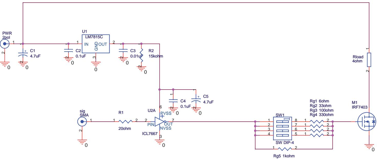
Figure C.1 – Schematic used to design the PCB.
