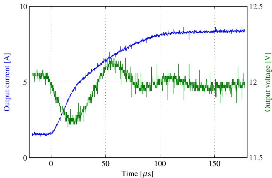
**Figure 6.11** – Load step response, 15% to 85% in 100μs.
