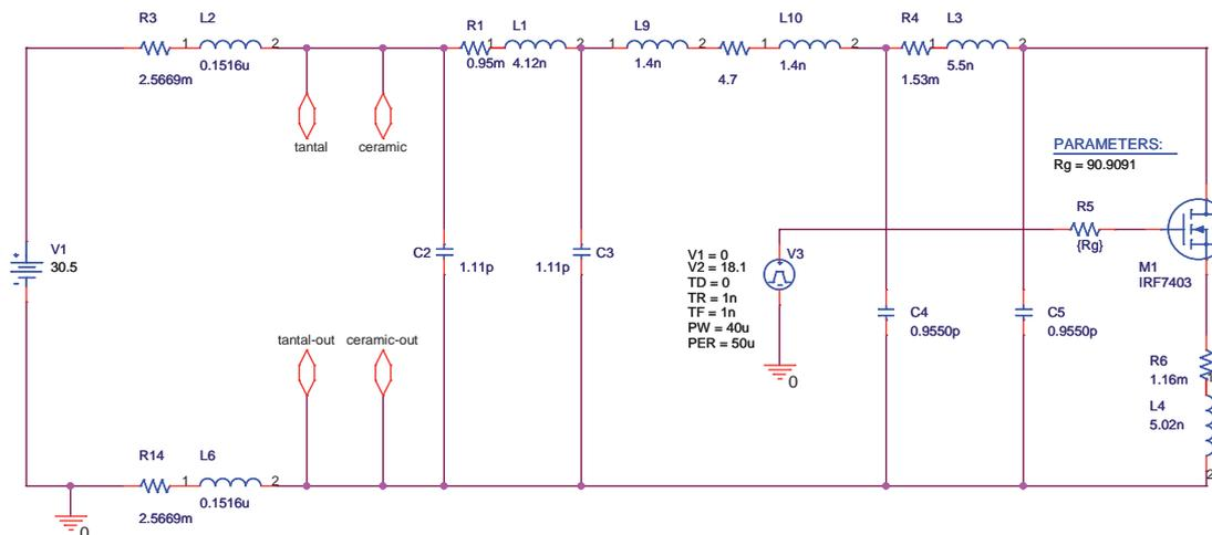
**Figure 5.4** – A more detailed model of TB1 including parasitic and stray components.
