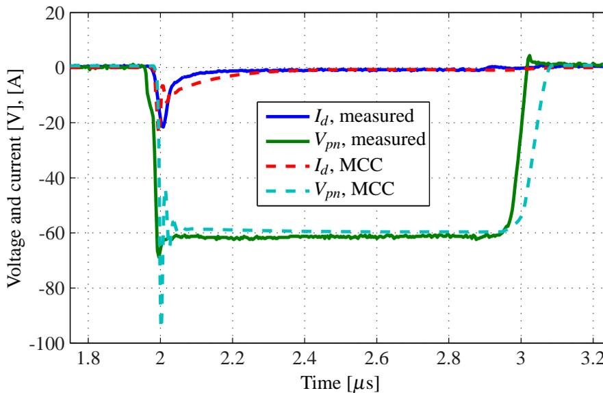
**Figure 6.7** – Measured and simulated drain current and diode voltage. The diode used during simulation is the implementation of the MCC diode model.
