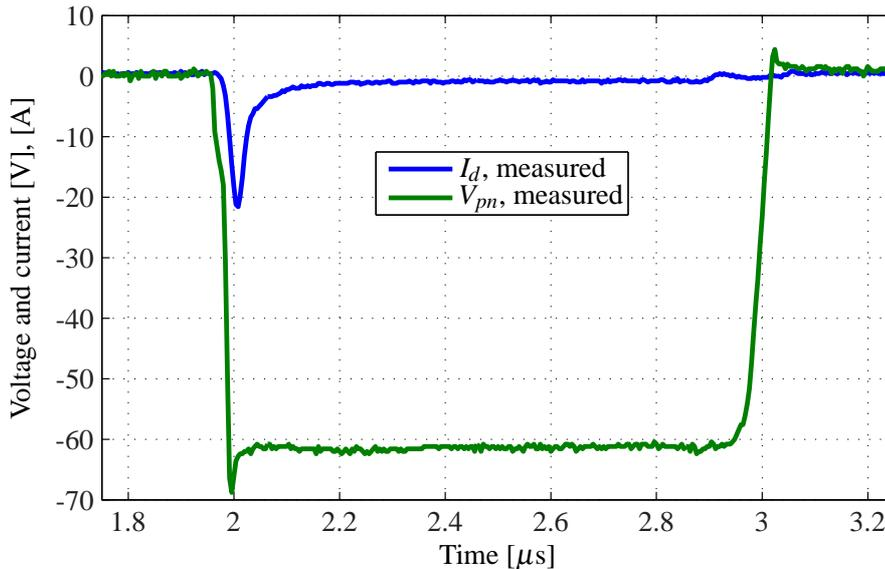
**Figure 6.3** – Measured MOSFET drain current and diode voltage.
