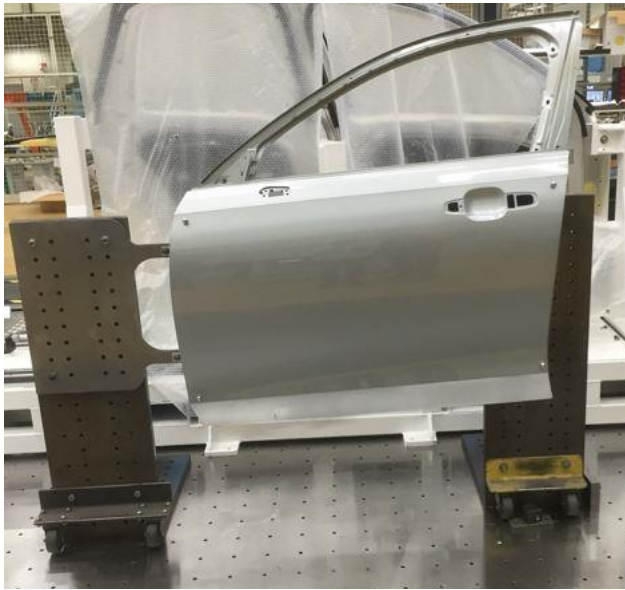
Figure 22. Fixturing of door
