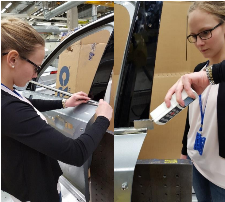
Figure 29. Left: Assembly of OWS. Right: Force estimation of assembly
