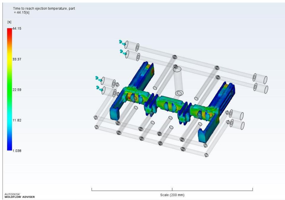
Figure 4.4: Time to reach ejection temperature with conventional cooling.
