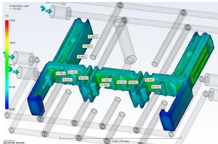
Figure 4.6: Temperature distribution on the part with conventional cooling.
