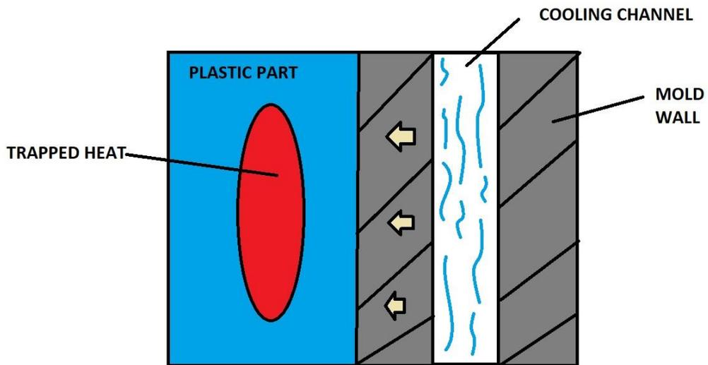
Figure 4.11: Representation of thickness effects regardless of cooling.
