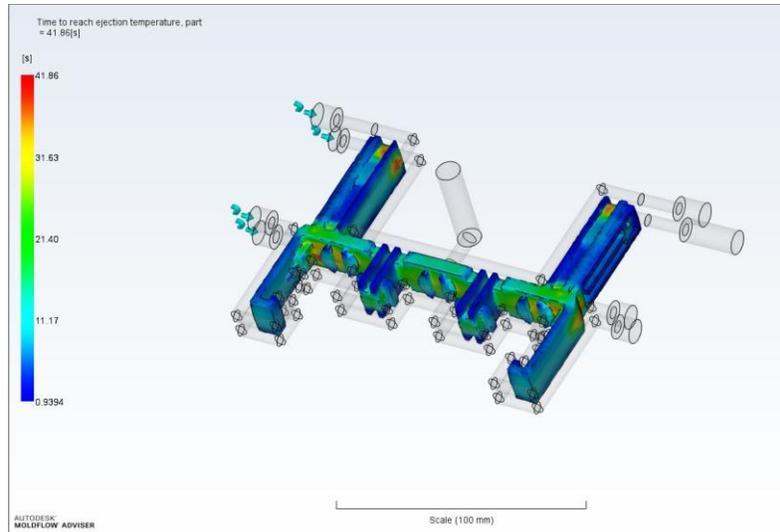
Figure 4.5: Time to reach ejection temperature with conformal cooling.
