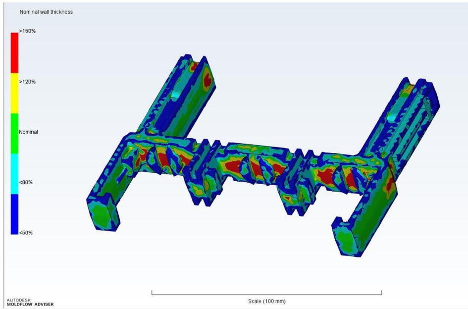
Figure 4.10: Deviations from nominal wall thickness
