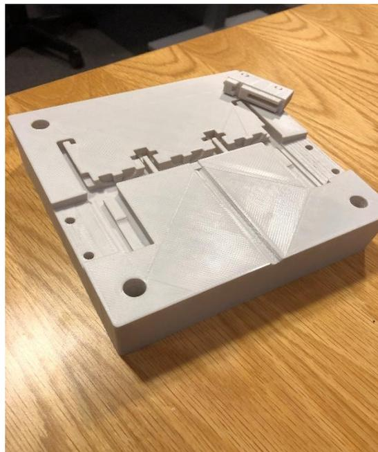
Figure 3.7: PLA model of the mold insert using Fused Deposition Modeling
