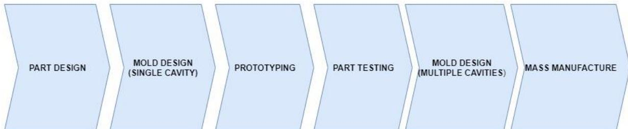
Figure 2.3: Process chain of the mold development process.
