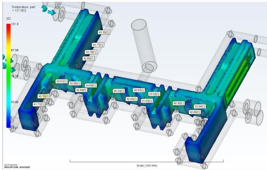
Figure 4.7: Temperature distribution on the part with conformal cooling.
