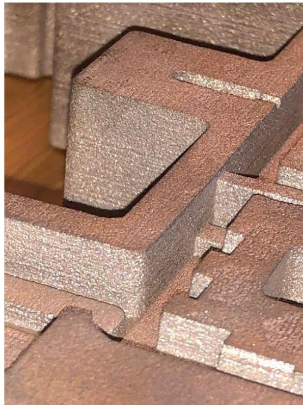
Figure 4.2: Surface roughness of the cavity.
