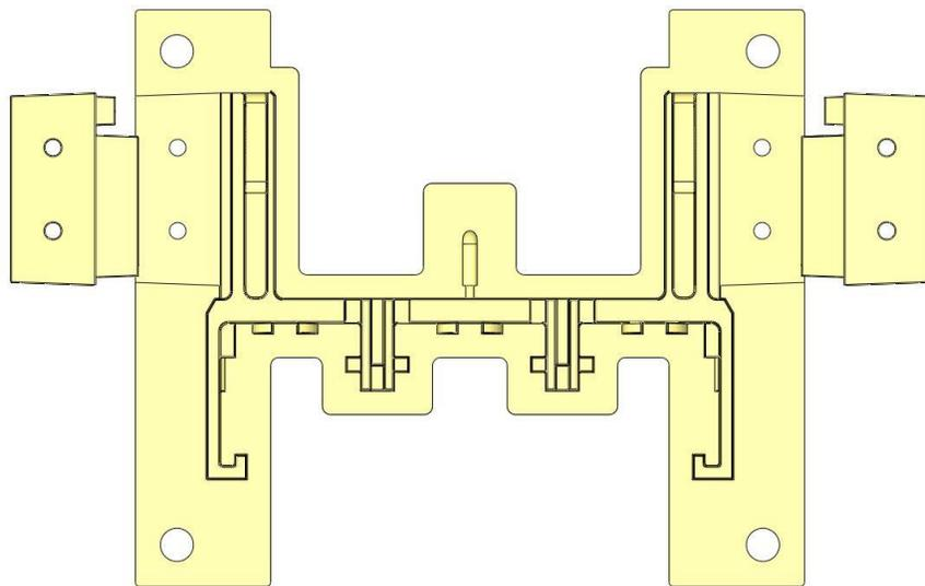
Figure 4.3: Design Iteration 3 for the binder jetting process
