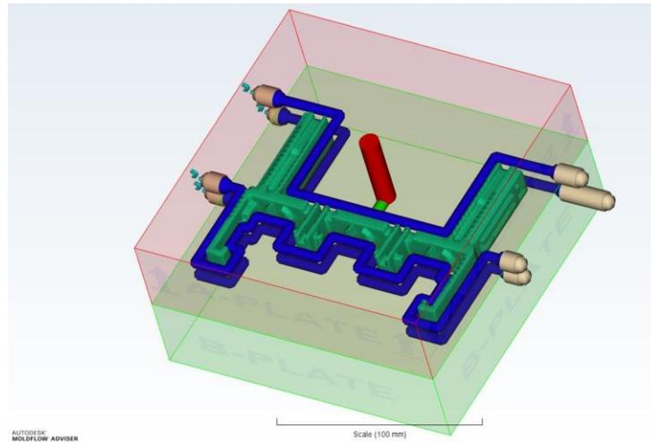
Figure 3.14: Conformal cooling channel design
