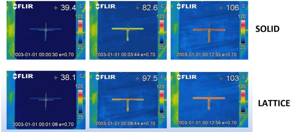
Figure 4.13: Infra-red images of the mold insert samples during heating
