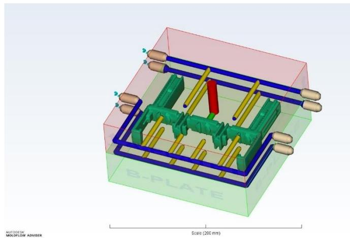
Figure 3.13: Conventional cooling channel design.
