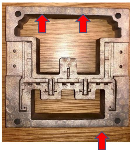
Figure 4.1: Failed part of the mold insert.
