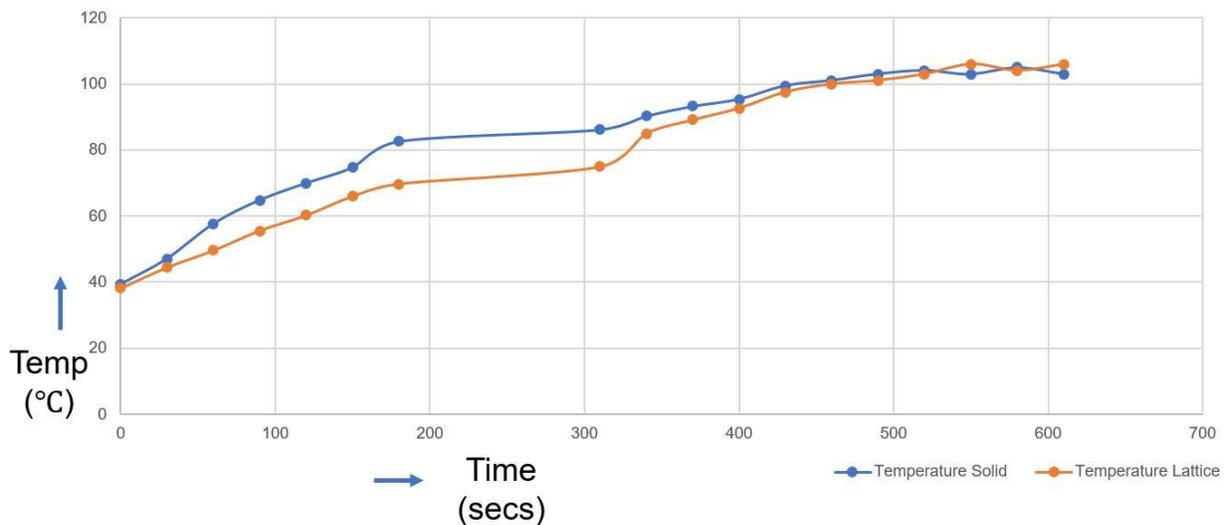
Figure 4.12: Time taken by the two mold samples to heat to 100°C
