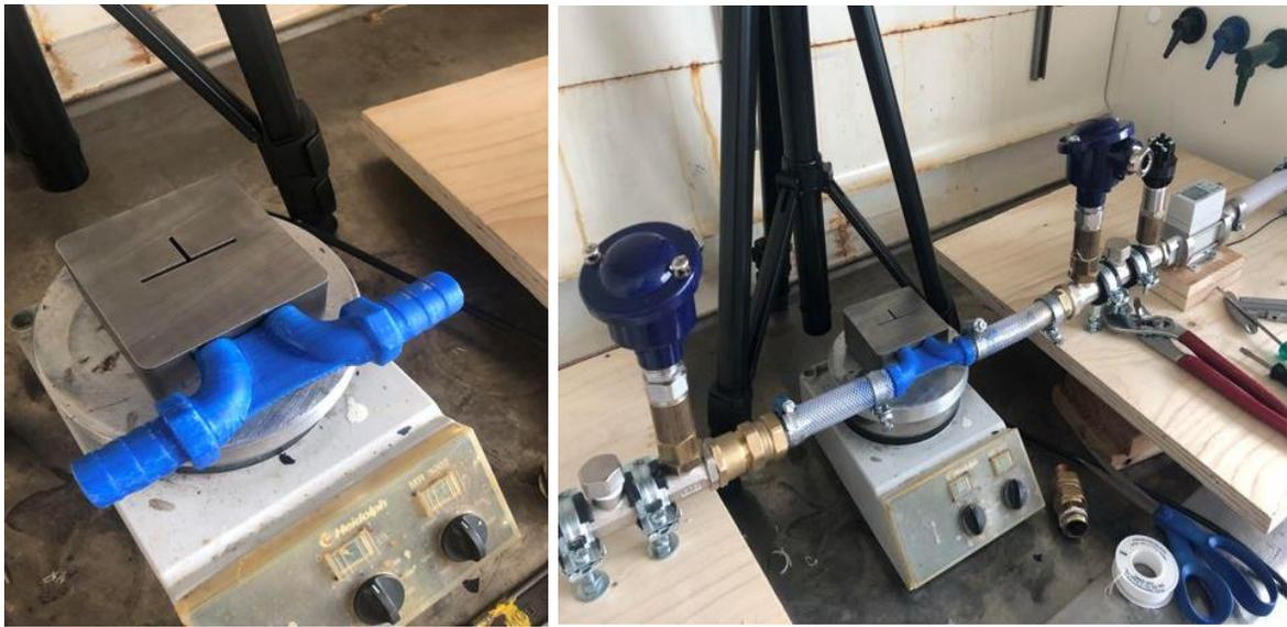
Figure 3.19: Water connection to the mold insert sample.
