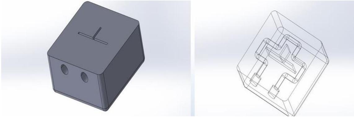
Figure 3.15: Sample of the mold insert with the cooling circuit.
