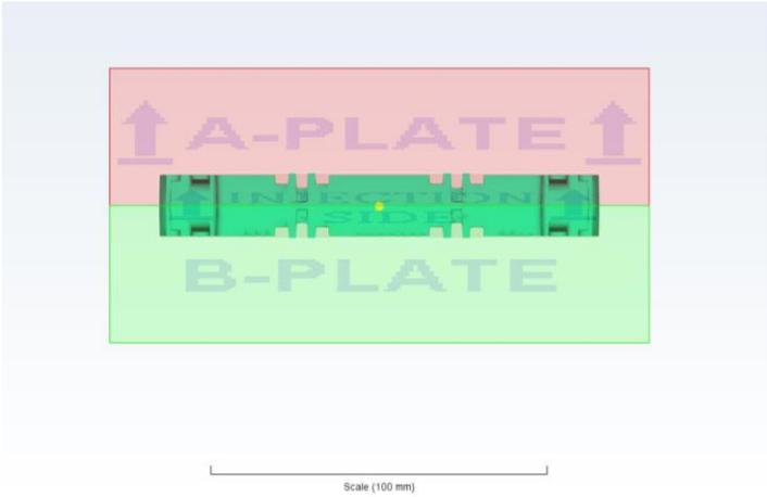
Figure 3.6: Parting line of the mold insert
