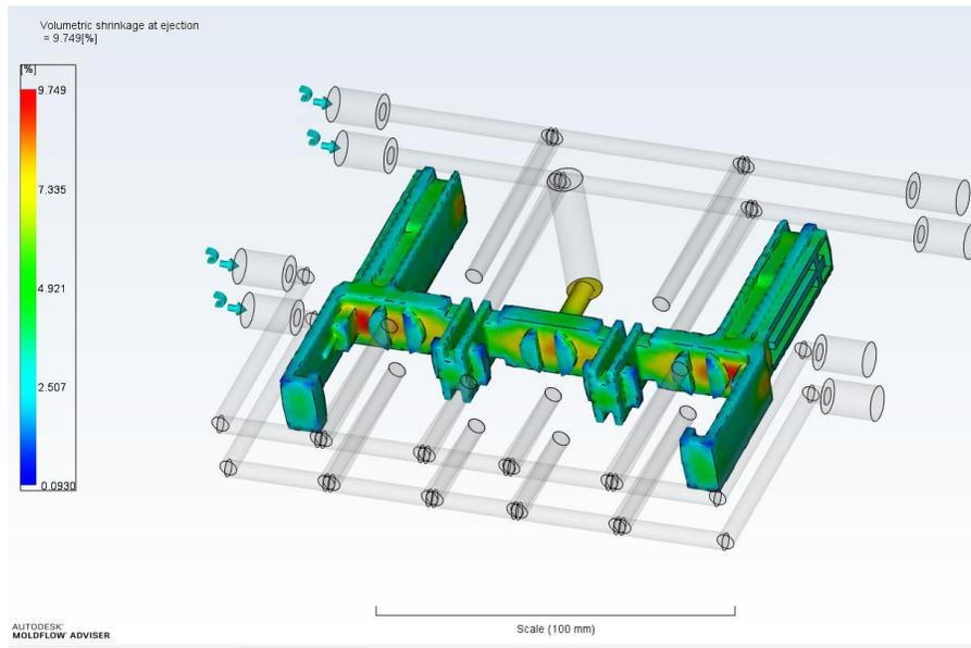
Figure 4.8: Volumetric shrinkage of the part with conventional cooling.
