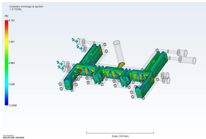
Figure 4.9: Volumetric shrinkage of the part with conventional cooling.
