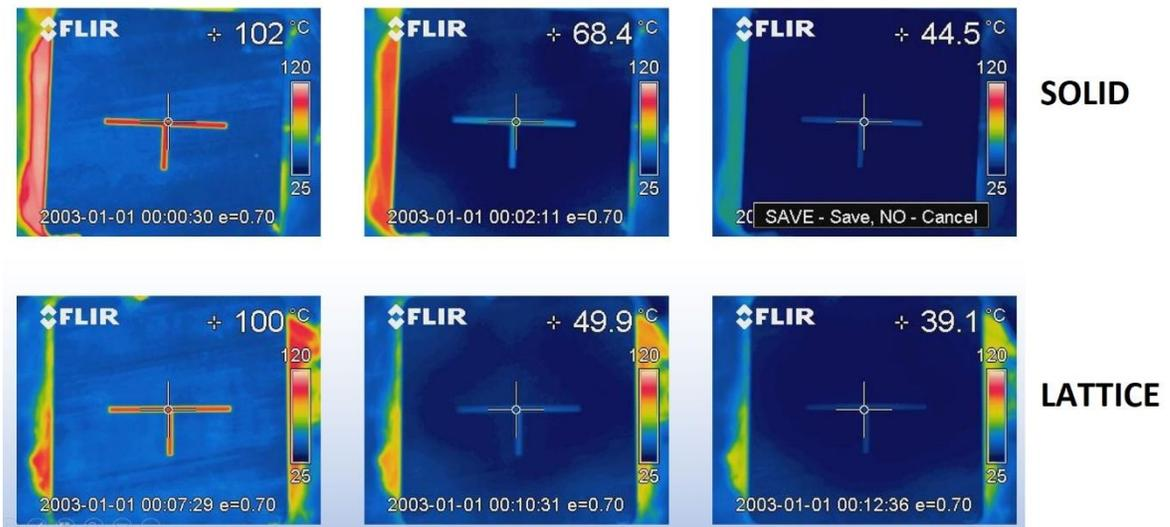
Figure 4.15: Time taken by the two mold samples to cool to 40°C
