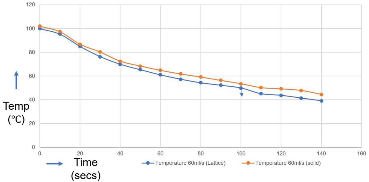
Figure 4.14: Time taken by the two mold samples to cool to 40°C
