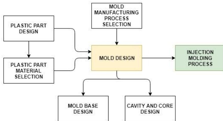
Figure 2.2: Factors influencing the mold development process [6].
