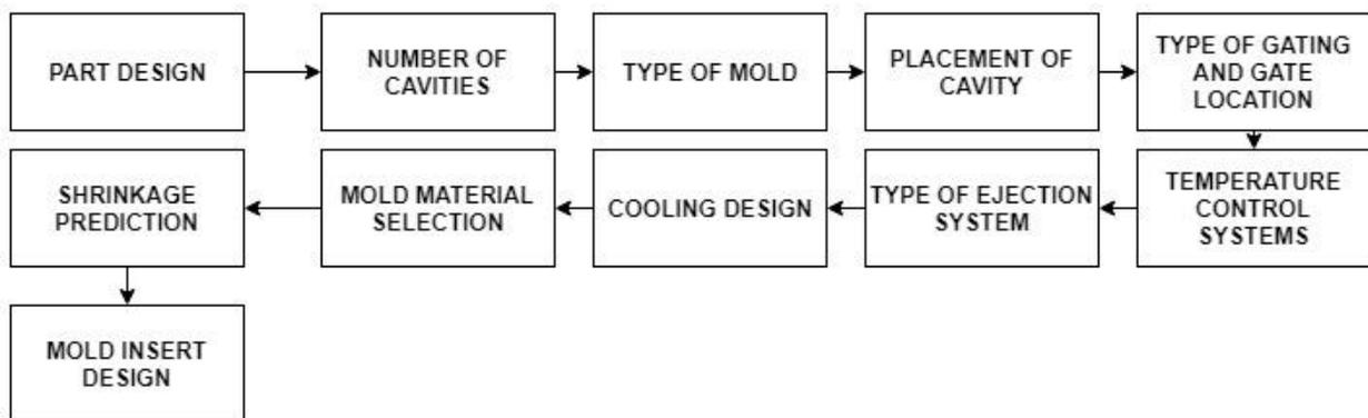
Figure 2.1: Stages of designing a mold insert [4].
