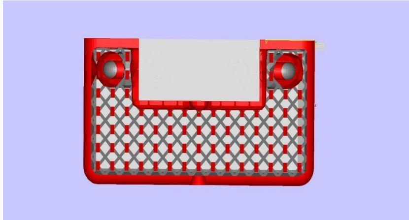
Figure 3.16: Cross-sectional view of the lattice structure mold insert
