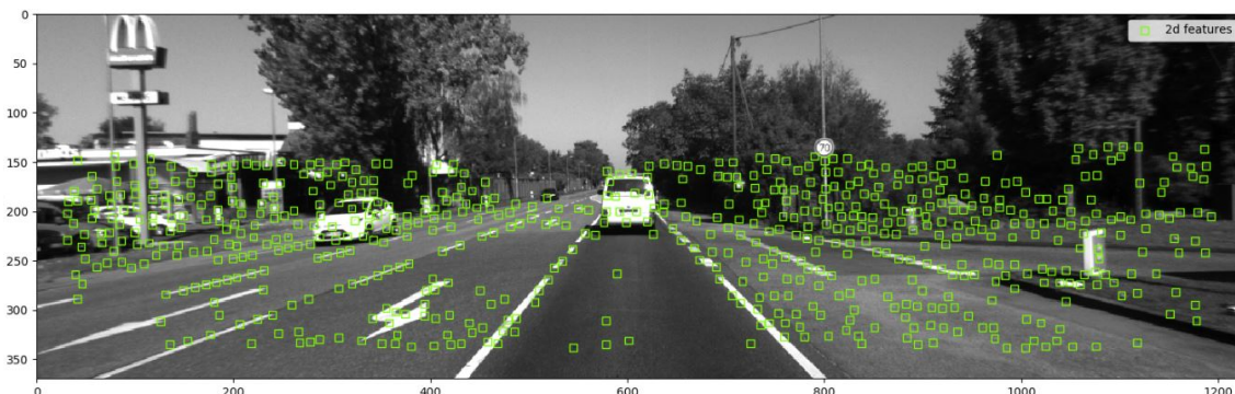
Figure 4.3: ORB feature extraction with SSC method (Green squares)
