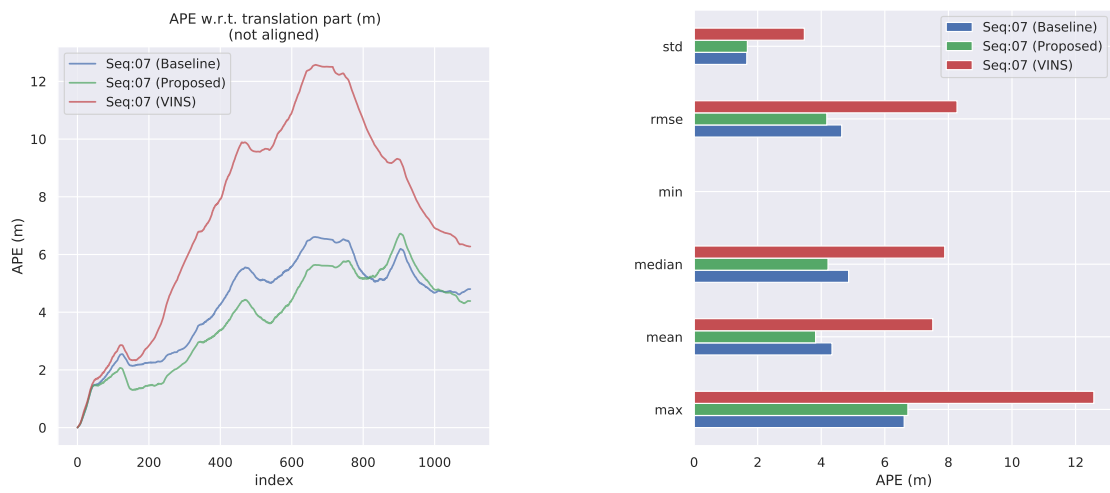
Figure 5.12: ATE comparison of VI-SLAM on KITTI sequence 07 under different gravity direction initialization methods (Baseline method, proposed AGI method and the method proposed by VINS-Mono)
