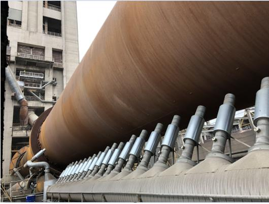
**Figure 2.5:** Picture of cooling air flow nozzle on the outside of the kiln
