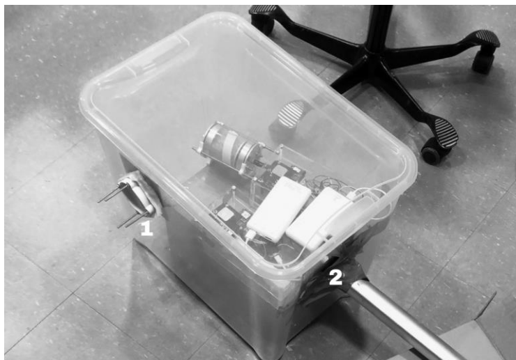
Figure 15. Box with filter, measurement devices and vacuum hose. Photo by authors
