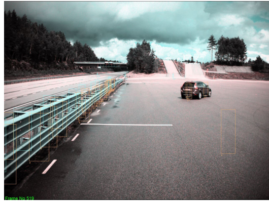
(b) Target moving away from guardrail trajectory.
