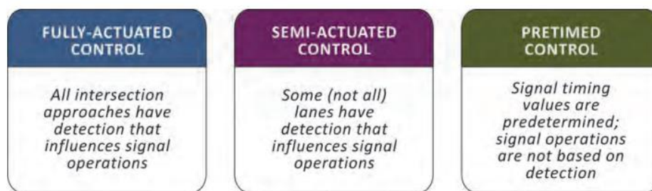
Figure 2.1: Different types of signal controllers (Fhwa, 2008)
