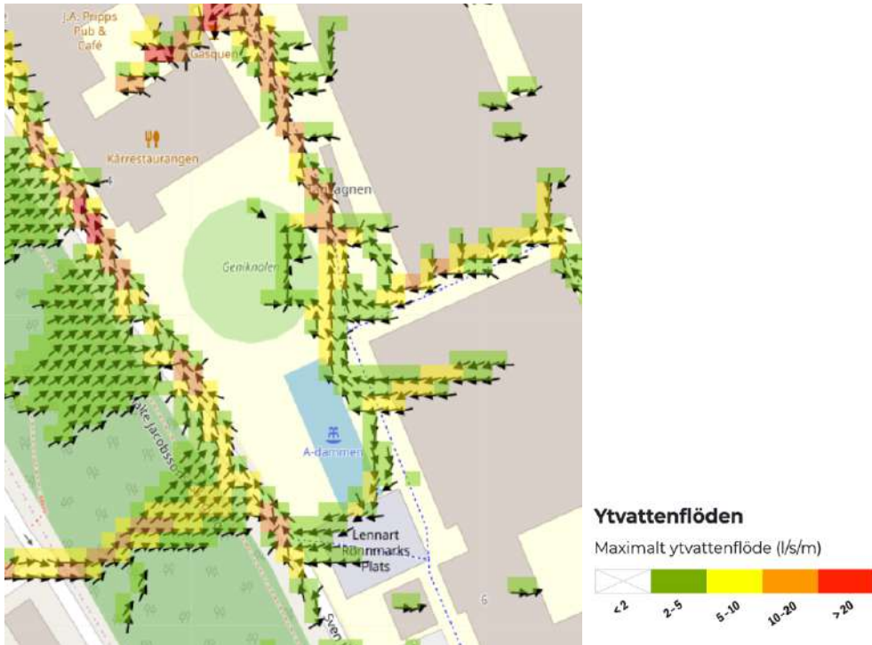
Figure 12. Water surface flow and direction in case of 100 year rain. (Göteborgs stad 2020)
